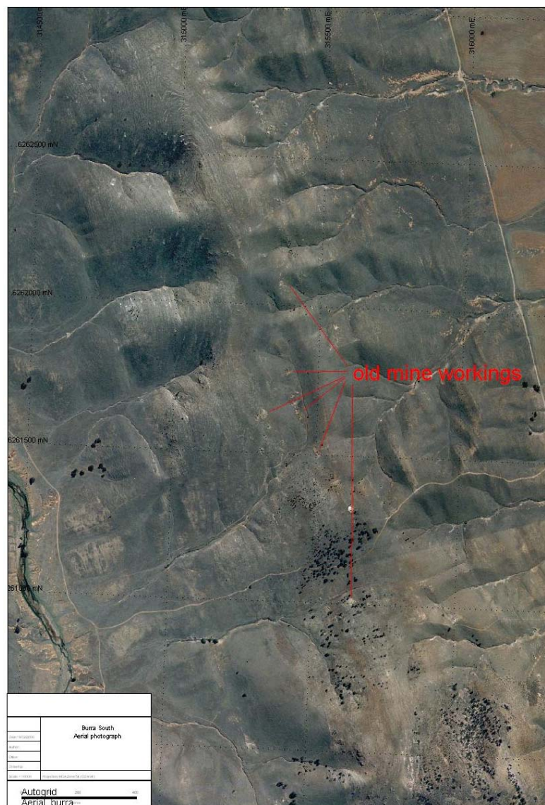
Figure 3. Aerial photograph of the Princess Royal prospect shows clearly all the old mine workings and trend of large structures like the plunging anticline.
