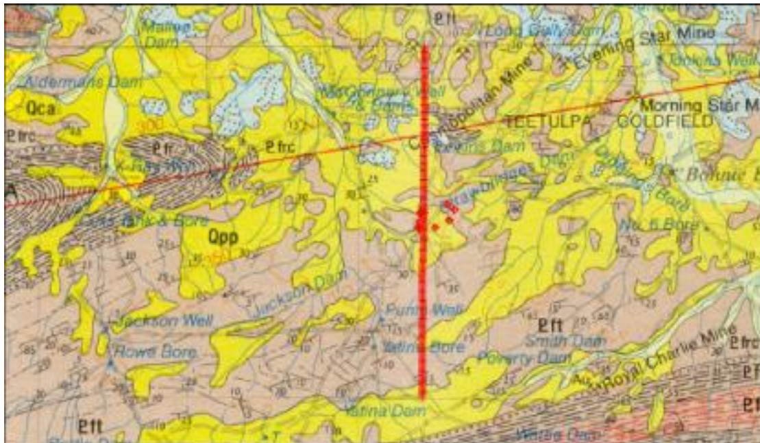
Figure 1 Location of the magnetic line for modelling and the location of preliminary exploration drill holes.
