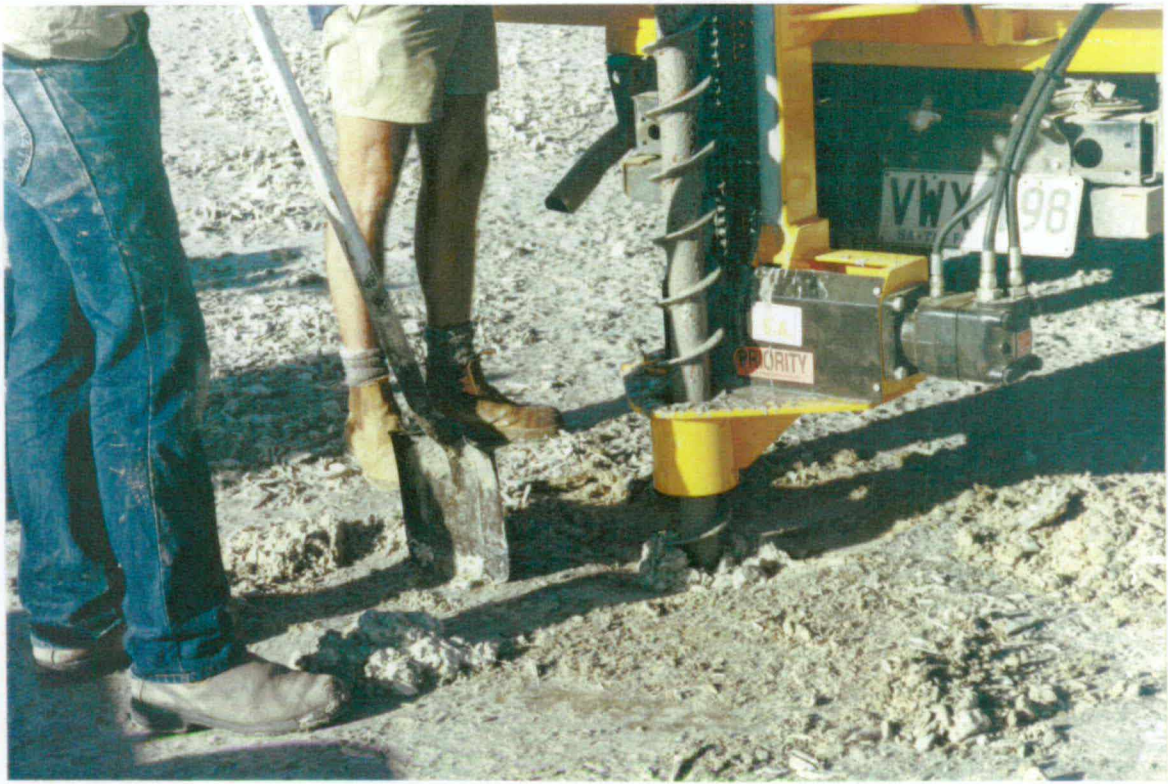
Plate 7: SOUTH MINE SITE February 1997 Machine auger rig after spudding in with white gypsarenite augering to the surface.
