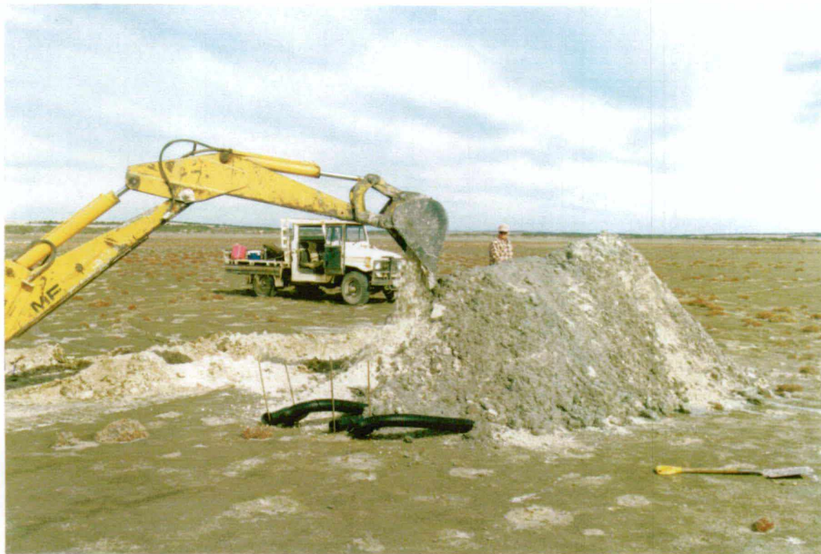
Plate 17 NORTH MINE SITE Stockpile K42 being established on folded black agri pipe. View South
