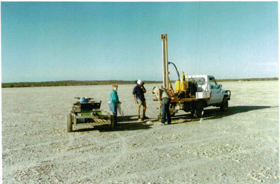
Plate 6: SOUTH MINE SITE February 1997 View south west at Hole K27. Sample of white gypsarenite being collected from 0-1m. Full sample bags are stacked on small trailer behind motor bike.
