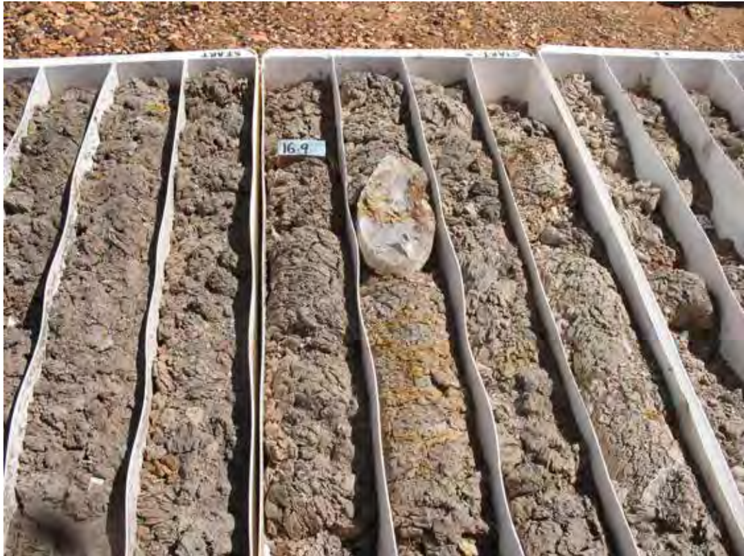
Photo 2.2 Weathered bulldog shale with gypsum in core
