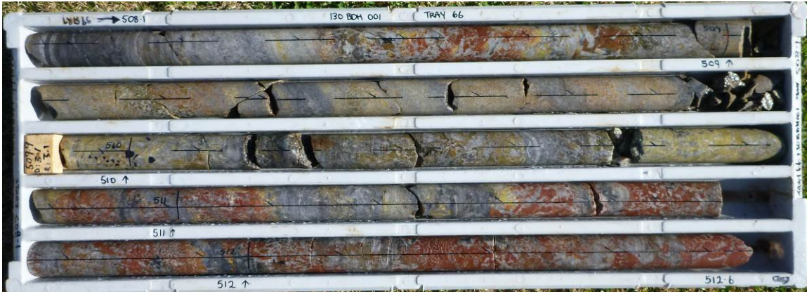
Figure 18: Example of mineralised iron flooding or alteration from 508-513m
