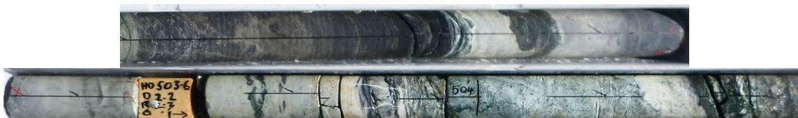
Figure 17: Example of mineralised carbonate veining from 503.4-504.4m
