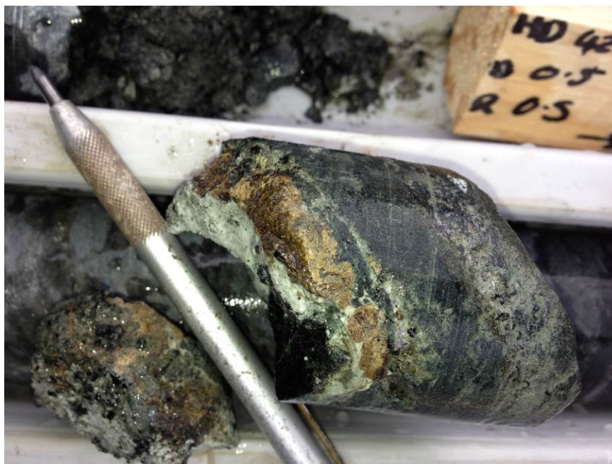
Figure 16: Orange-yellow Sphalerite vein
