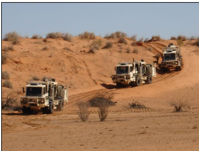
Plate 2: Vibrator trucks traversing a seismic line
