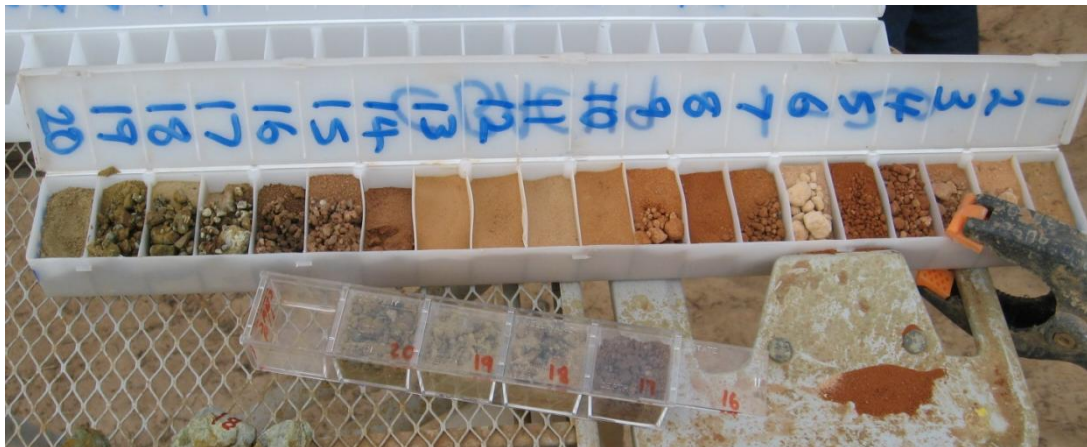
Figure 4: Typical chip tray showing ~15m of shallow cover
