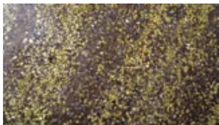
Core from Angas Zinc Project drillhole AN29; this section assayed 27.7 m at 2.8% Pb, 12% Zn and 19 g/t Ag; width of view is ~90 mm (courtesy Terramin Resources). (Photo 400951)
