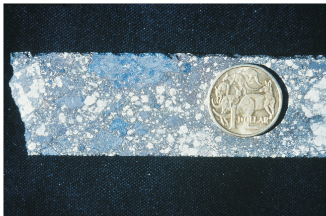
High-grade bornite–chalcocite mineralisation hosted by haematite–granite breccia. (Photo 48176)
