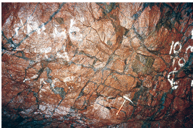
Weakly brecciated Roxby Downs Granite. The breccia matrix primarily consists of sericite and haematite, and occupies steep dilated joints and crosscutting fractures. (Photo 48170)
