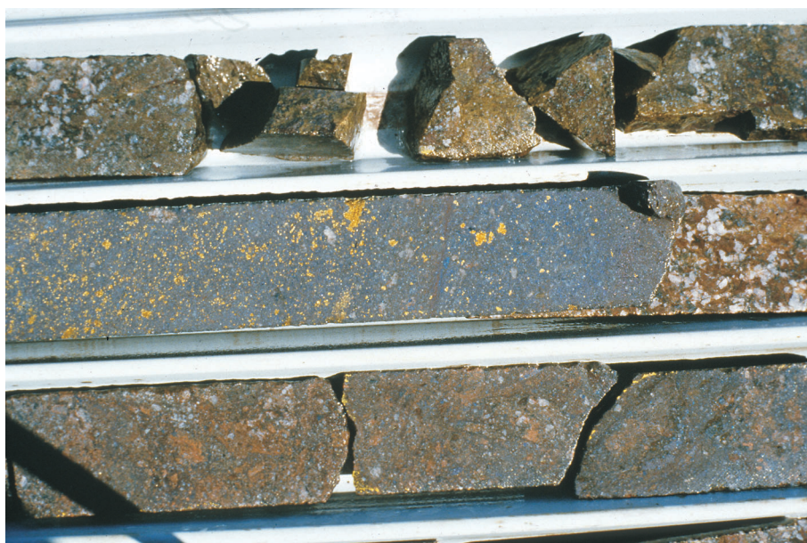
Disseminated mineralisation in drill core showing the chalcopyrite–bornite sulphide transition, almost in the centre of the image and marked by a faint brown line. (Photo 48178)
