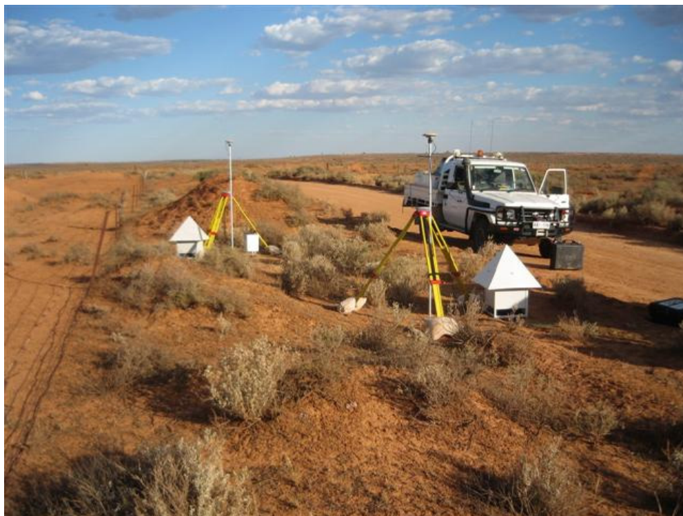
Photo 11: Post process GPS base setup north of Morgan
