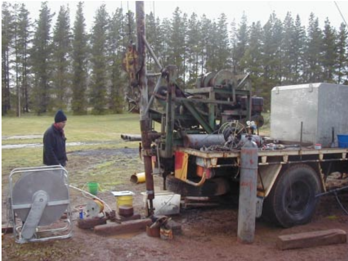
Plate 3 Pole truck and air tanks used to install inflatable packers into the well and green (Fluorescein) discharge water. (photo 047940)
