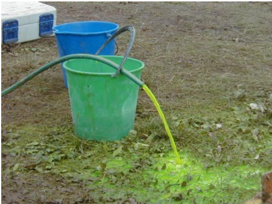
Plate 4 Fluorescein in groundwater discharge during first recovery cycle. (photo 047941)
