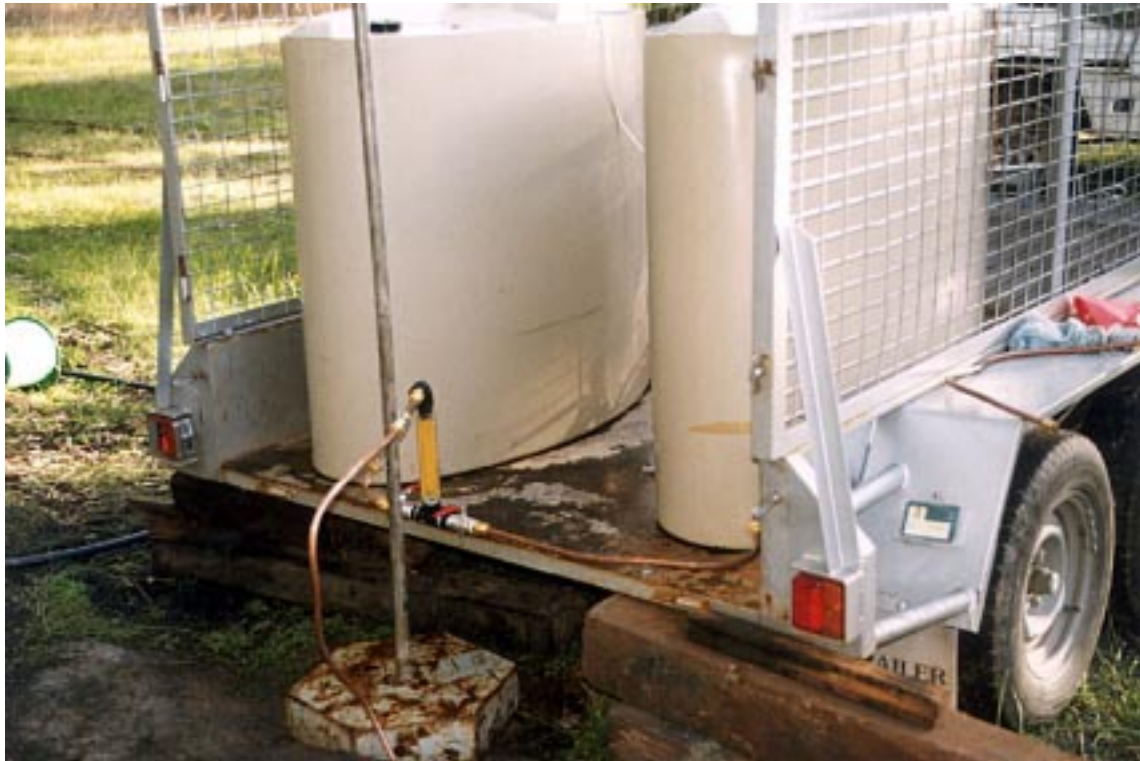
Plate 1 Two rainwater tanks, copper tube, T-piece and flow meter used for the injection phase, ASR trial at Wendouree Winery. (photo 047939)
