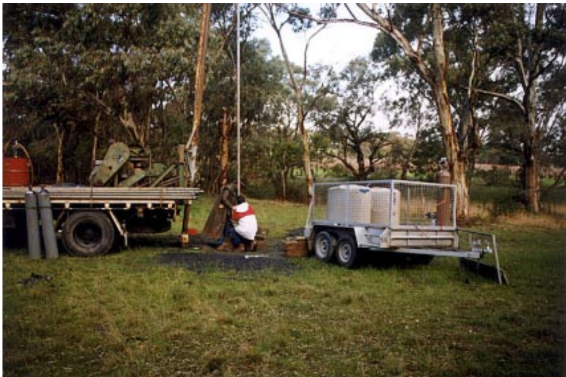
Plate 2 Installation of inflatable packers with pole truck and two rainwater tanks; one containing tracer solution (He and Br) and the other being chaser (bore) water, field site for ASR trial at Wendouree Winery. (photo 047938)
