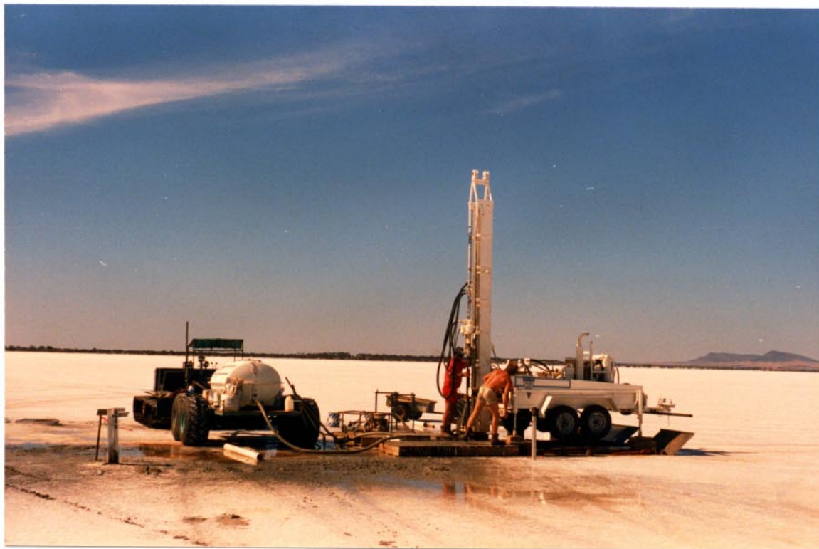
1. Diamond Drill modified for transport over salt lake.
