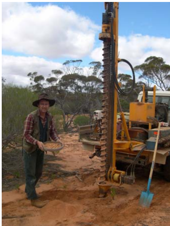
Fig 15. 4WD-mounted soil auger rig used for calcrete sampling. Geologist shown holding sieved sample of nodular calcrete.
