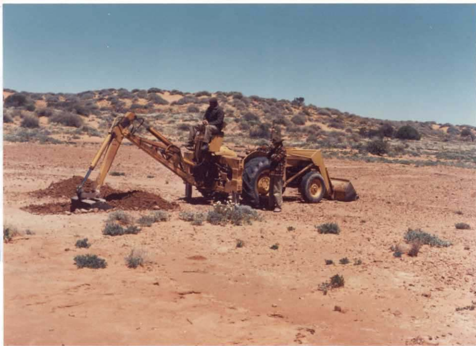
Fig. 3. Backhoe in operation (October, 1978) Mapping in areas masked by thin cover is greatly facilitated by use of a backhoe. Looking for the contact of the Marree Formation and the 'Stuart Creek Beds' at BHT 42A1.
