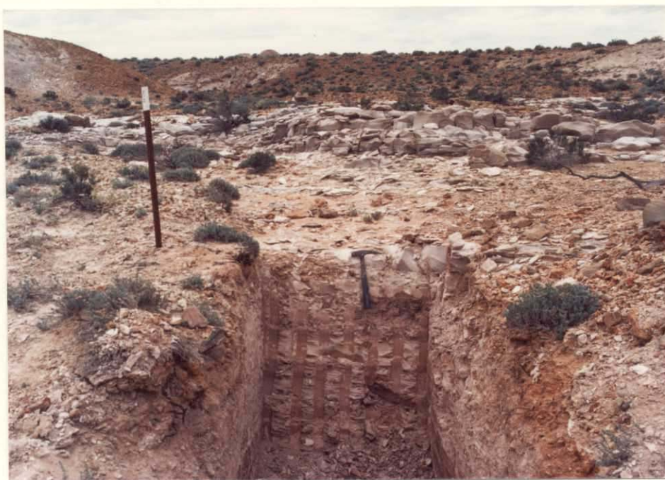
Fig. 4. Bunyerroo Formation (October, 1978) "Kopi" - mud contact in Bunyerroo Formation at BHT 39. Bleached white/grey mudstone ("kopi") overlies soft, moist, pink, fissile mud. Marree Formation is present in BHT 39B on the horizon.
