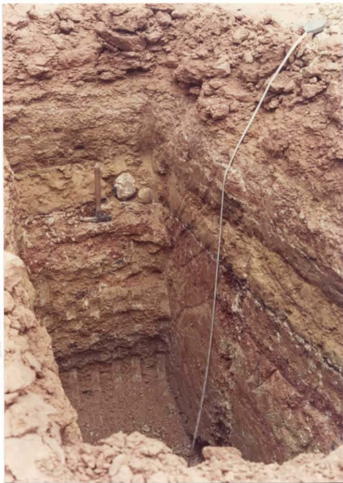
Fig. 15. BHT 27 (October, 1978) Sand of the Mount Sarah Sandstone with lag cobbles (near hammer) at the base overlies mud of the Marree Formation. (See log of BHT 27 in Appendix A).
