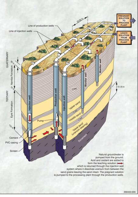
Fig. 3 Schematic ISL wellfield (courtesy Southern Cross Resources).
