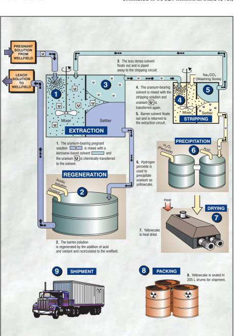
Fig. 4 Schematic uranium solvent extraction plant (courtesy Southern Cross Resources).
