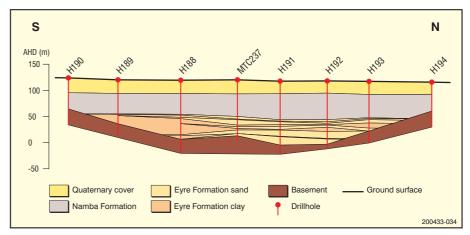
Fig. 2 Cross-section of the Yarramba Palaeochannel.
