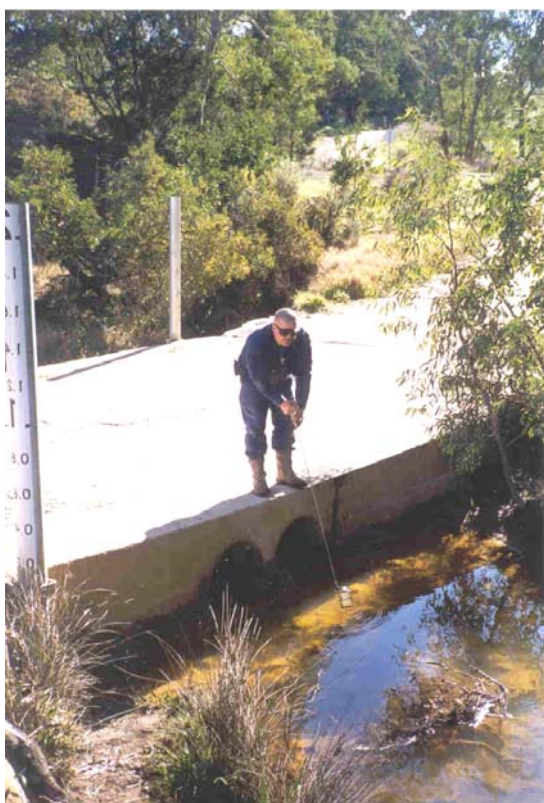
Figure 10. Grab sampling of creek water for chemical analysis at Melbourne Bridge.
