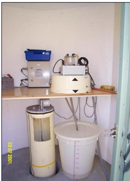
Figure 8: Automatic flow data recording and composite water sample collection equipment located in the monitoring huts.
