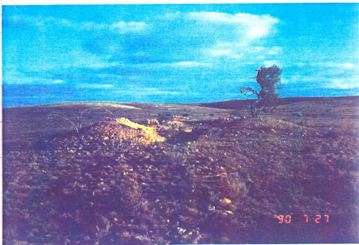
Sta. 97. View south. Mullock heap to right accumulated through hand sorting, possibly some screening, of copper/gold ore. It is inconceivable to think that the miners here were unaware of the high gold and silver values associated with these copper ores.
