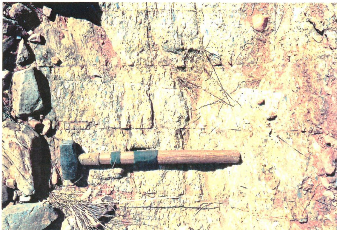
Photo 02. Station 05. View vertical. Top of photo S60°E. Shows sheared conglomerate, hammer parallels jointing: 210/90, 5/m. Fracture cleavage coincides with shearing: 112/85SW.
