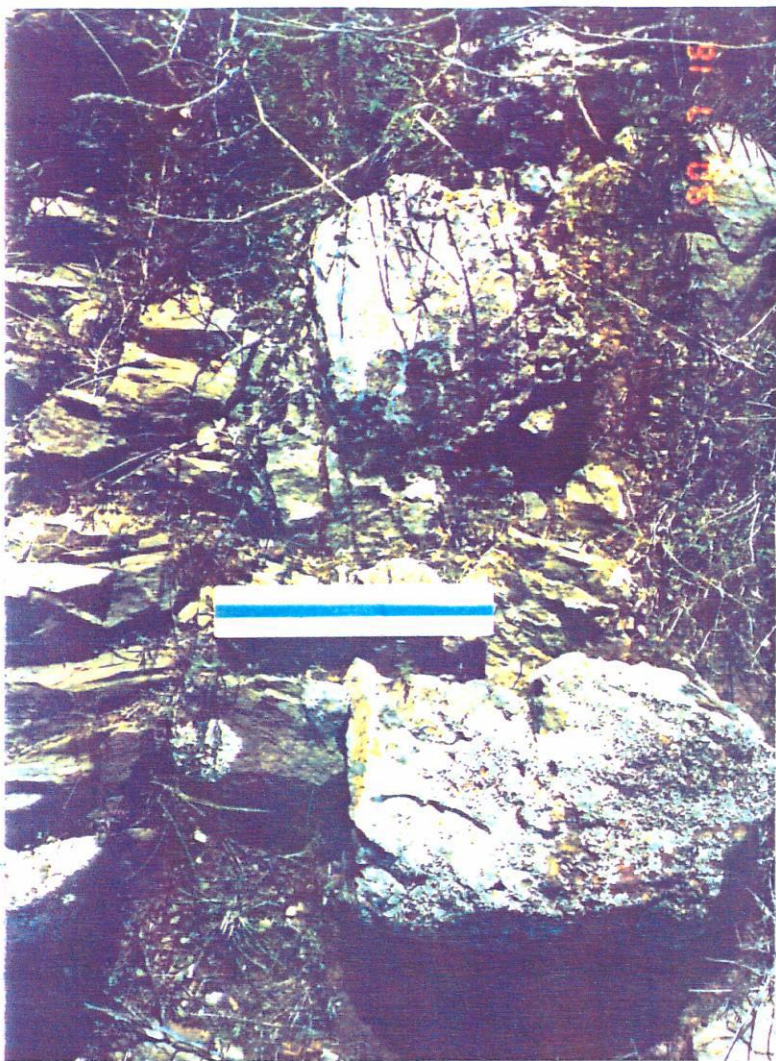
Sta. 40. Intermediate dike intruding siltstone 40-60 cm thickness, 05/85NW. Sample MO 05R (Au .002 ppm, Cu 65, Pb 52, Zn 22, Ag <1). View 165°
