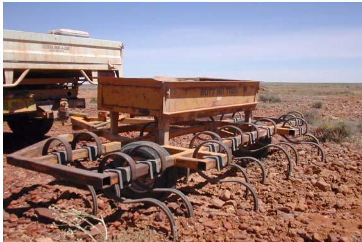
Figure 3: Specially designed scarifier that was used for the rehabilitation
