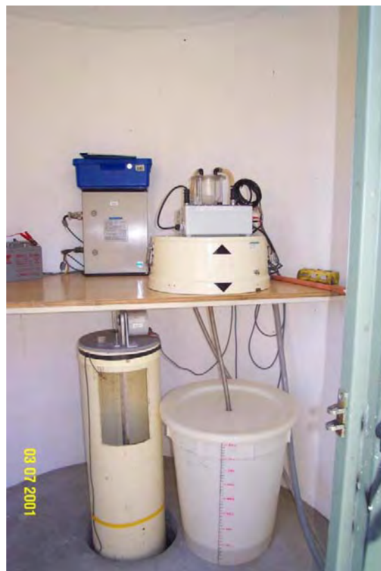
Fig 8. Automatic flow data recording and composite water sample collection equipment located in the monitoring huts.
