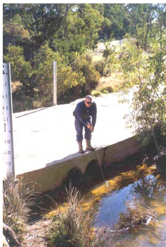
Fig 10. Grab sampling of creek water for chemical analysis at Melbourne Bridge.
