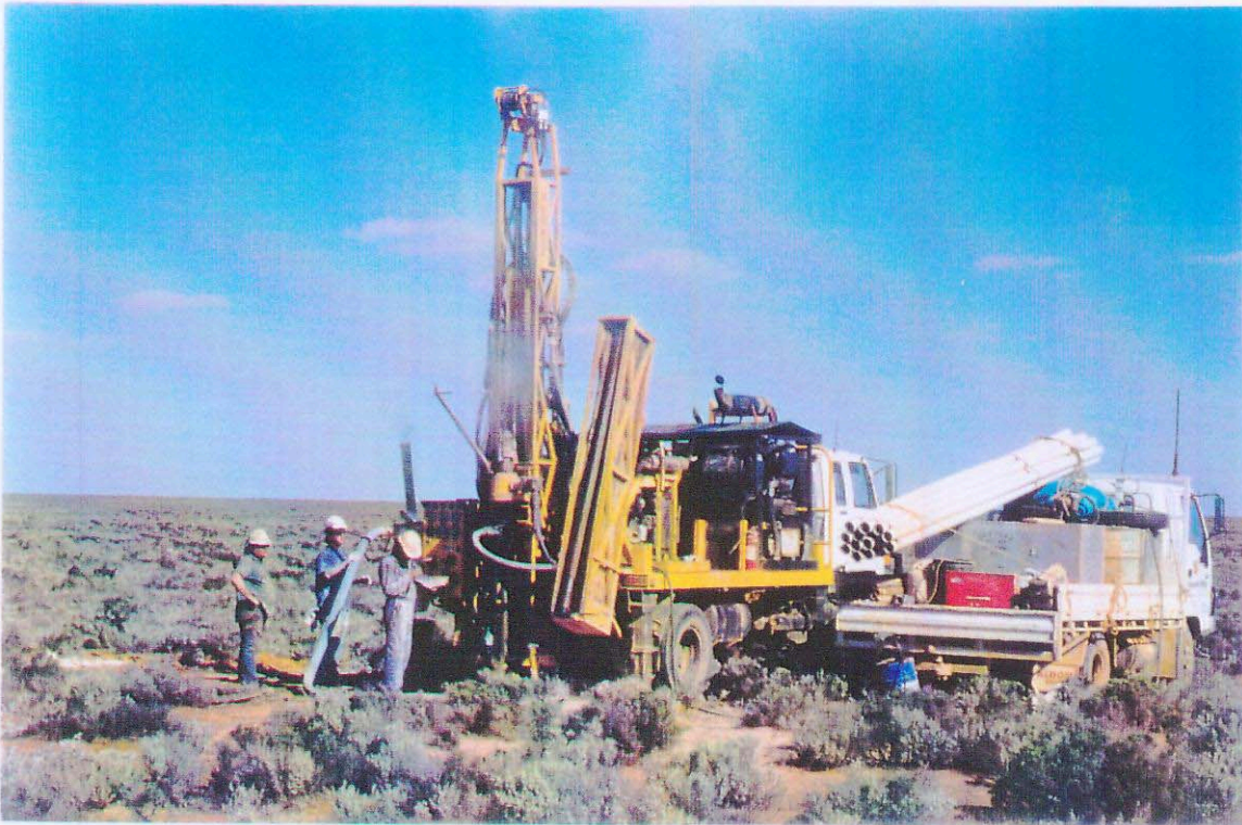
Plate 1: Johannsen Drilling RAB/aircore drilling rig and support/water truck, OS-1 prospect, EL 2012.
