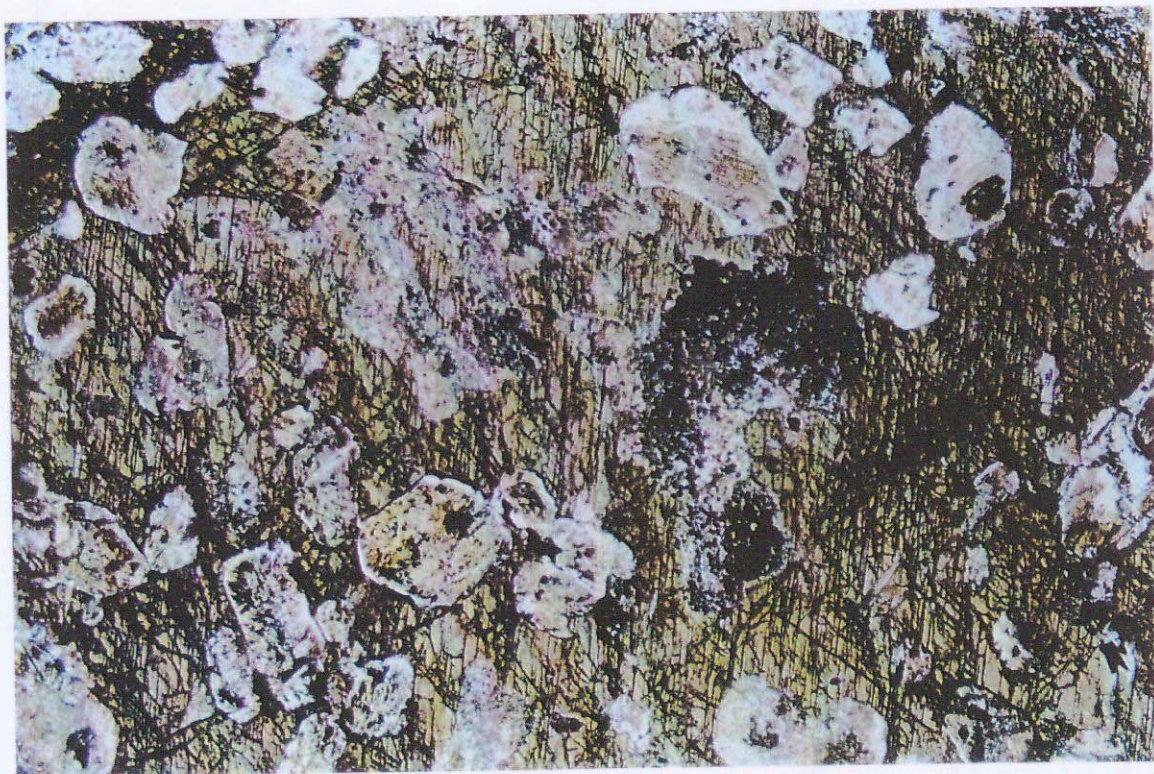
Fig 8 40213 green 0.45 mm TS. OL. Further example of coarse poikilitic hornblende ( green ) studded with altered small crystals of ex-pyroxene.
