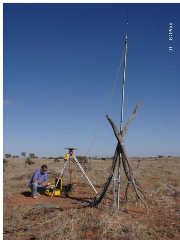
RTK GPS base station showing UHF link to mobile Base station coordinating unit and power supply and Wence holding the controller. A similar setup is in the vehicle.
