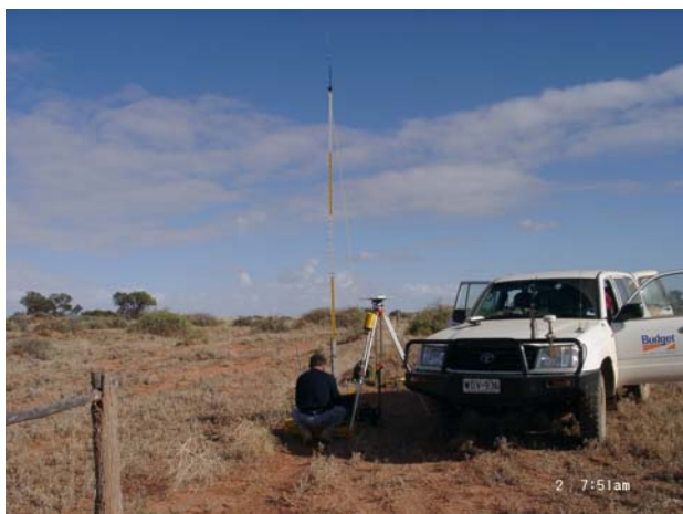
Reading the La Coste Romberg gravity meter .
