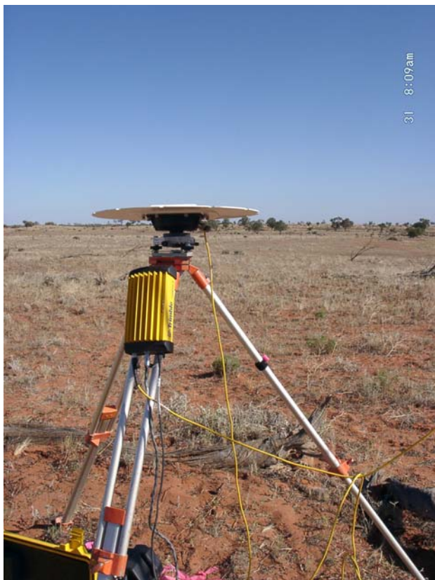
RTK GPS base station showing GPS receiver
