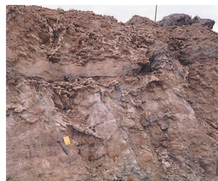
Graphite ore in the plasmic weathering zone extensively re-cemented by groundwater carbonate. (Photo 47520)
