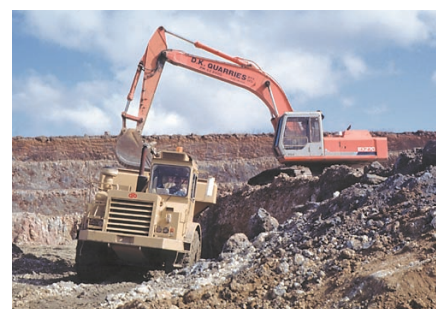
Loading graphite ore by bucket excavator at the Uley Mine. (Photo 47521)
