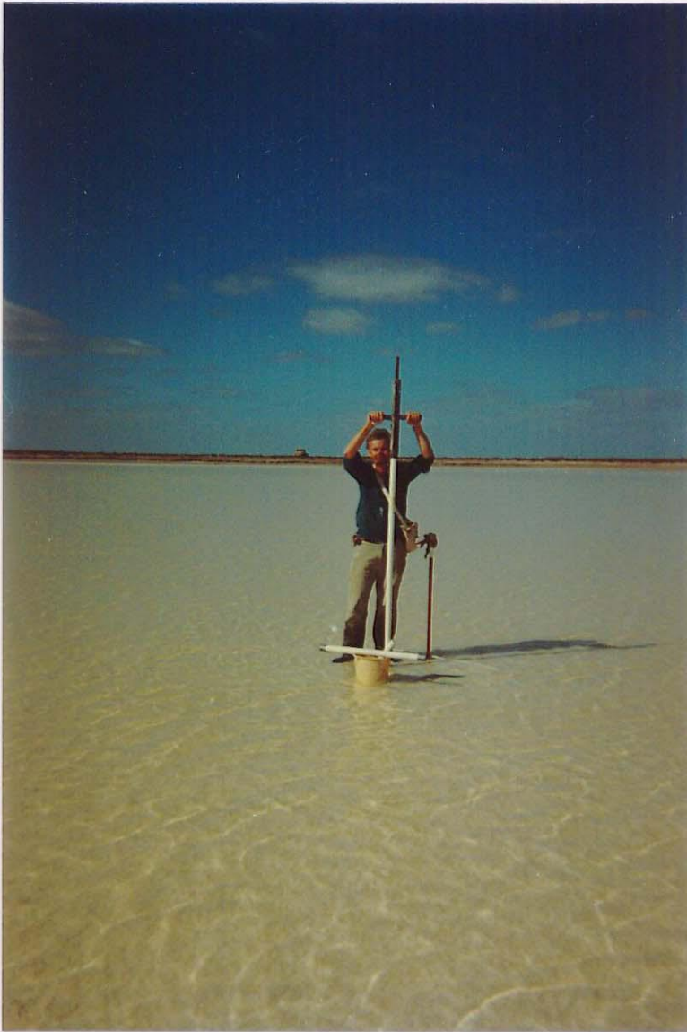
PLATE 1 - PUSH TUBE CORING, COOKE PLAINS EMBAYMENT Sean Kennedy operating coring device at Hole CP12. April 1990
