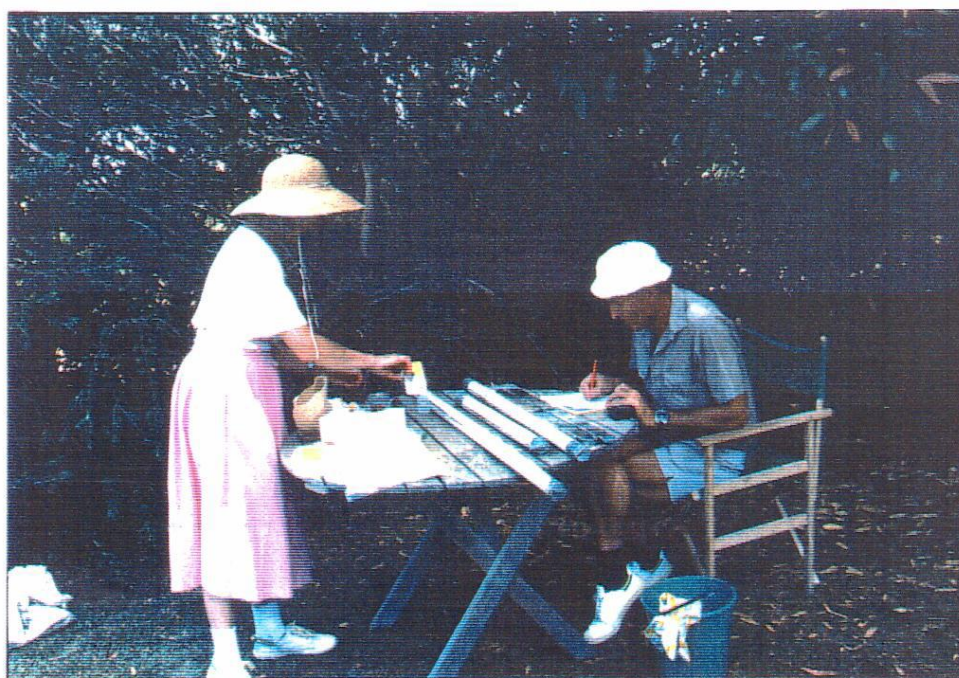
Plate 13 Logging and sampling. February 1992. Split core is logged lithologically and half core is bulked over appropriate intervals and submitted for chemical analyses.
