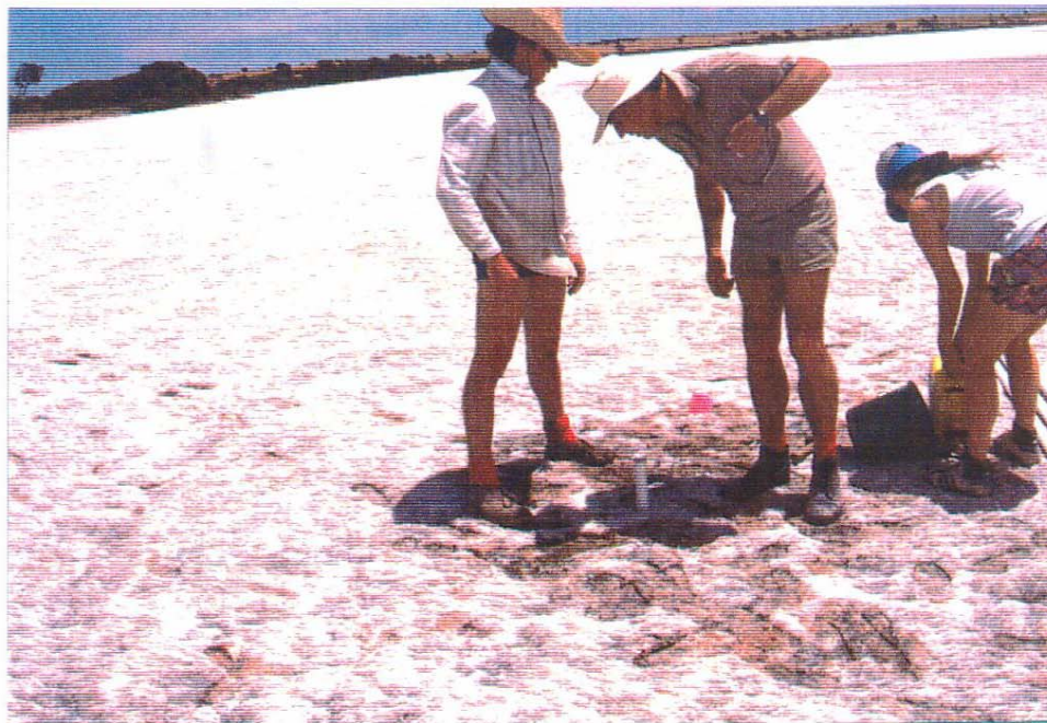
Plate 7 WARNES - completion of first length of PVC tube. January 1992. Hole WS40. Tube is filled with water and rubber bung inserted.
