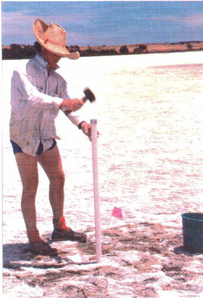
Plate 6 WARNES - PVC tube being hammered January 1992. Hole WS40. Aluminium dolly in top of tube and numbered pin marker used to identify each hole.
