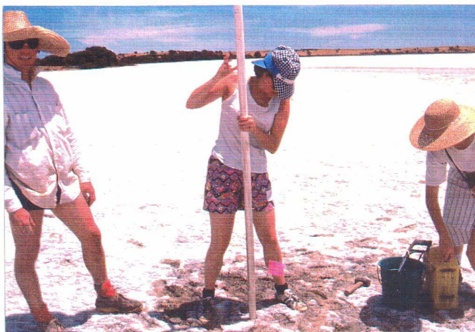
Plate 8 WARNES - extraction of PVC tube full of gypsum. January 1992. Hole WS40.
