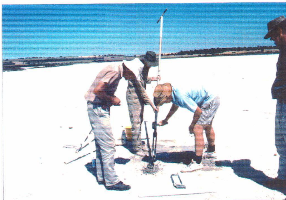
Plate 10 LIHOU - removing sample from hand auger February 1992. Hole L9. Hammering gypsum out of slotted auger tube.
