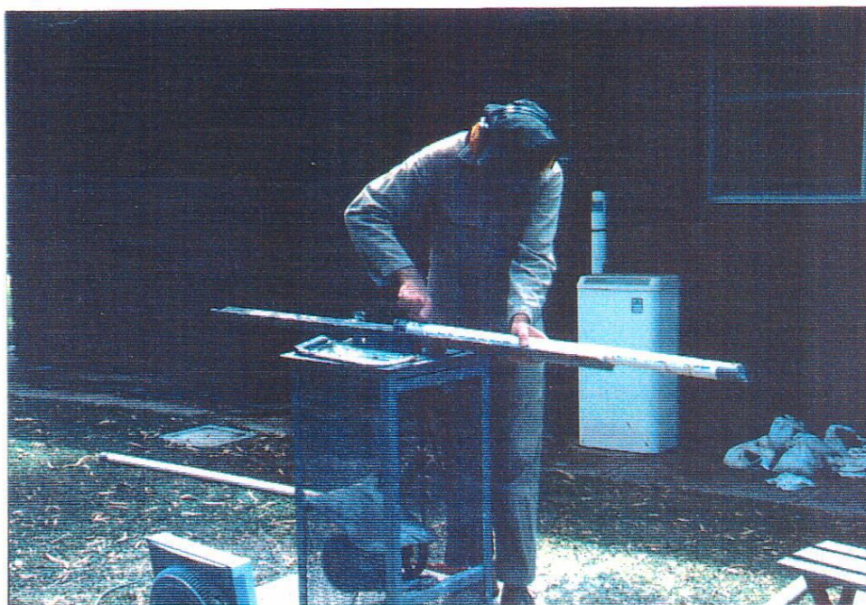
Plate 12 Splitting PVC tube. February 1992. A wire splitting device is pulled through the sawn tube thereby splitting the core sample in half.
