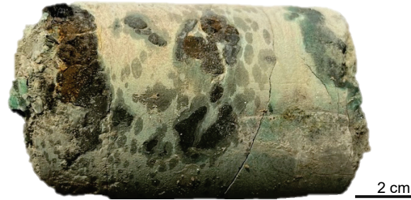
Malachite staining and manganese oxides. Tapley Hill Formation at 98 m from CW006RD 6 (Windabout deposit)
