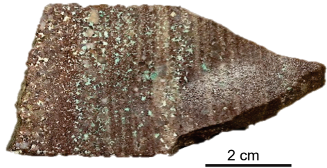
Red Sandstone with micro cavities infilled with clays. Whyalla Sandstone at 17.7 m from 840/670 (House deposit)
