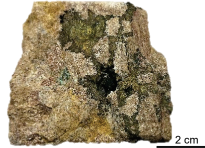
Limonite with chalcocite-chalcopyrite-bornite crackle veins. Pandurra Formation at 35 m from M350-250 (Cattlegrid deposit)
