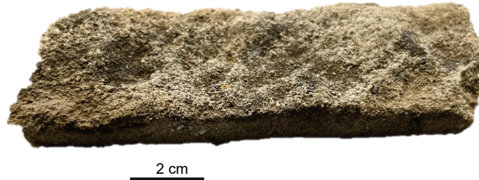
Soft sandstone with disseminated manganese oxides. Whyalla Sandstone at 68 m from LW 60 (Windabout deposit)
