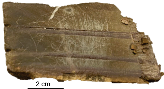
Micro sulphides and oxidized sulphide veins. Tapley Hill Formation at 32.4 m from MG 23/2 deposit (Mg14 deposit)
