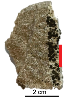
Muscovite and chalcocite vein. Whyalla Sandstone at 28 m from 820-750 (Gun deposit). Red line representing the closeup of the photo below
