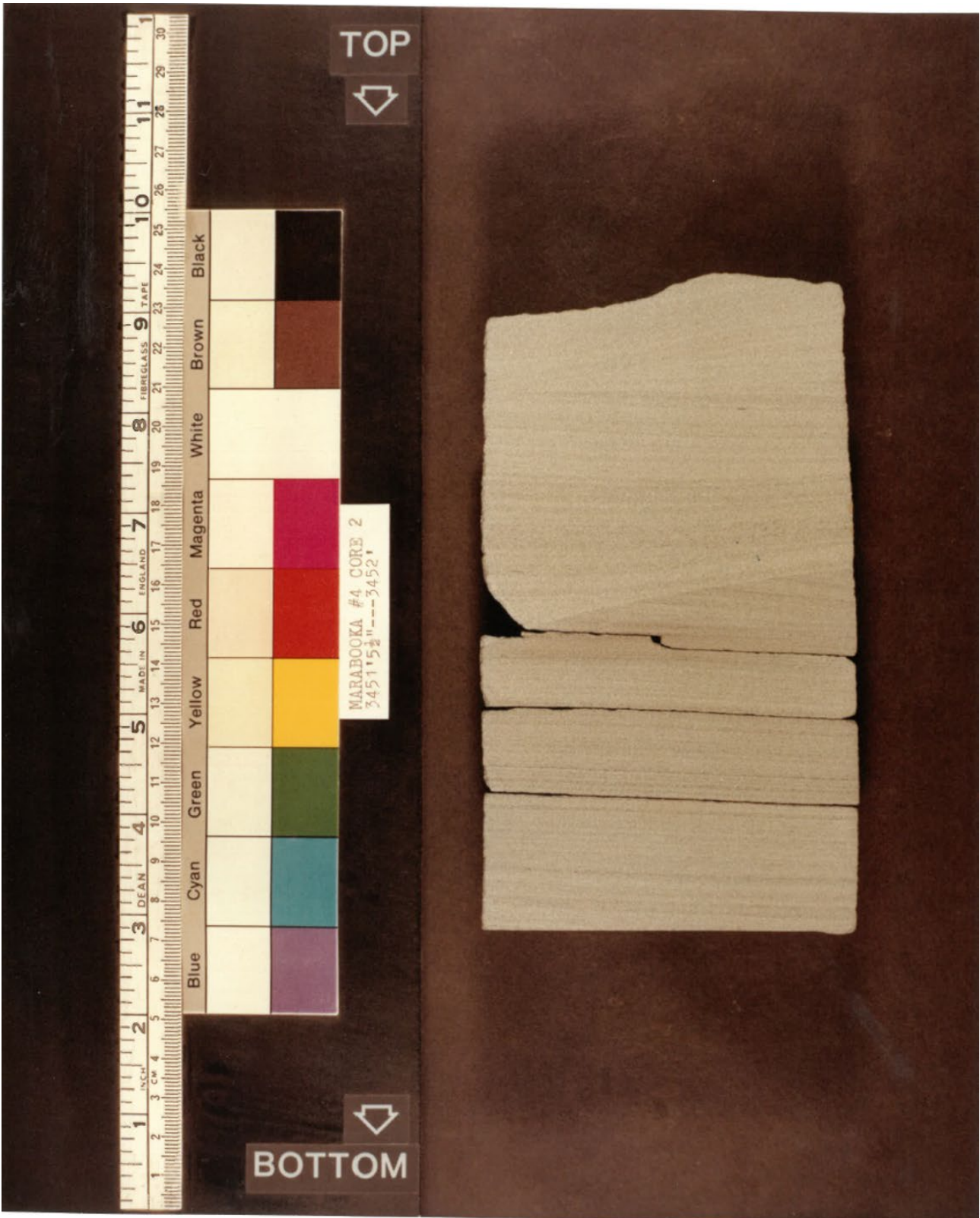
Figure A3.11 Coorikiana Sandstone lower cycle slabbed full hole from core 2, 3451' 5 1/2'' – 3452' (driller's depth).
