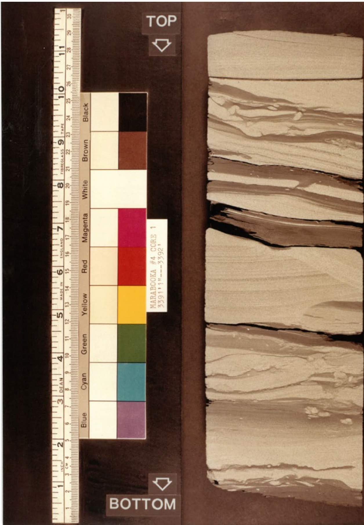
Figure A3.2 Coorikiana Sandstone upper cycle slabbed full hole core 1, 3391' 1" – 3392' (driller's depth).
