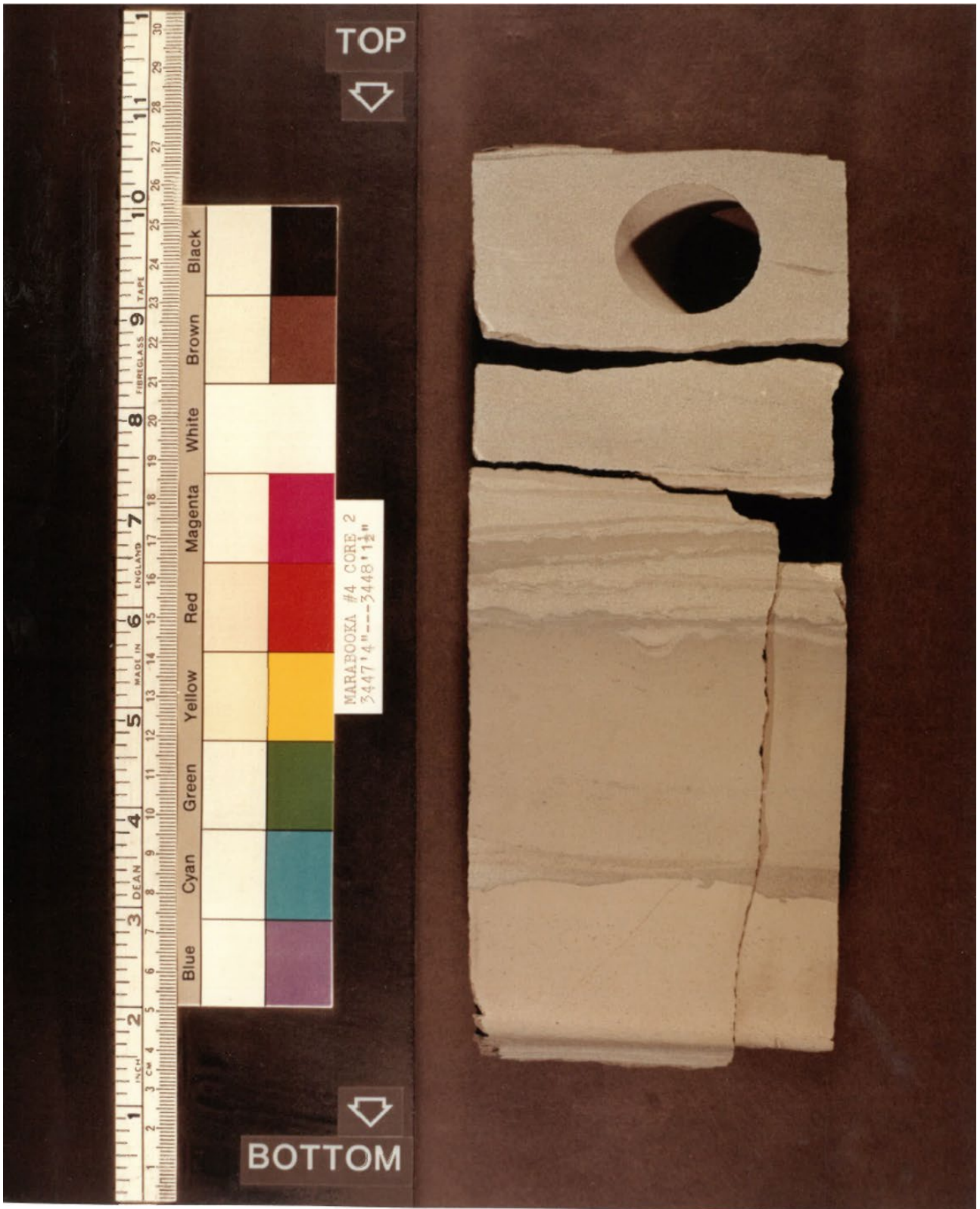
Figure A3.10 Coorikiana Sandstone lower cycle slabbed full hole from core 2, 3447' 4" – 3448' 1 1/2" (driller's depth).
