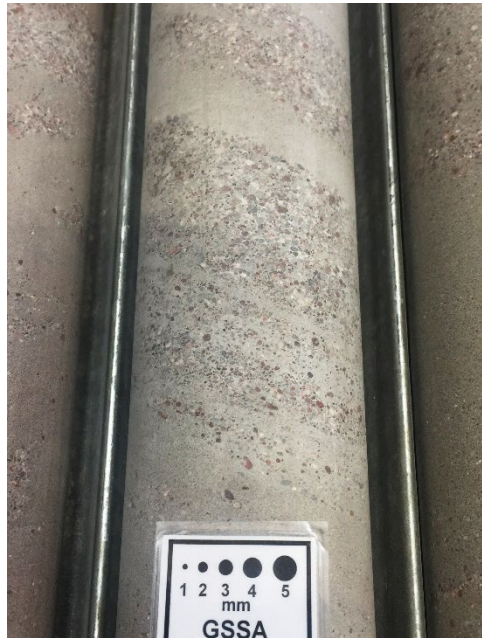
planar bedded fine- to coarse-grained sst
