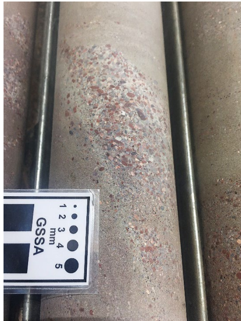
'floating' coarse-grained sandstone patches
