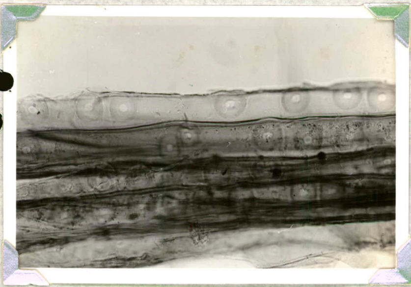
A. Tracheidal Wood fragments showing large bordered pits. x400. Core 14 at 8563 ft.
