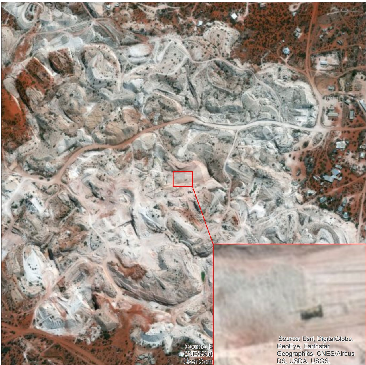
Figure 9. A bulldozer works a large area in the heart of the Old Field, indicating significant unmined areas within previously worked ground.
