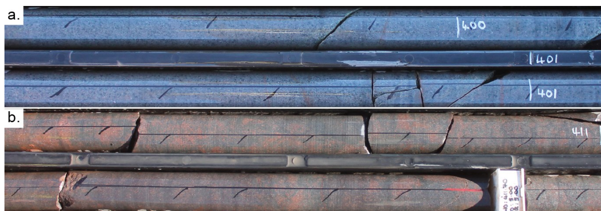
Figure 13. Representative core photos of microgabbro. a) 399.3–401.4 m: porphyritic, with thin hematite veins, and b) 409.2–415.3 m, with abundant pink patches representing felsic melt segregations.
