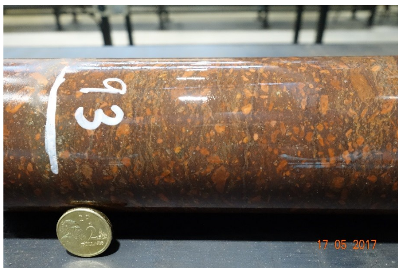
Brecciation (possible fine autobreccia) and more altered sporadically from 95 m – see core photo at 95.1 m (below) .
