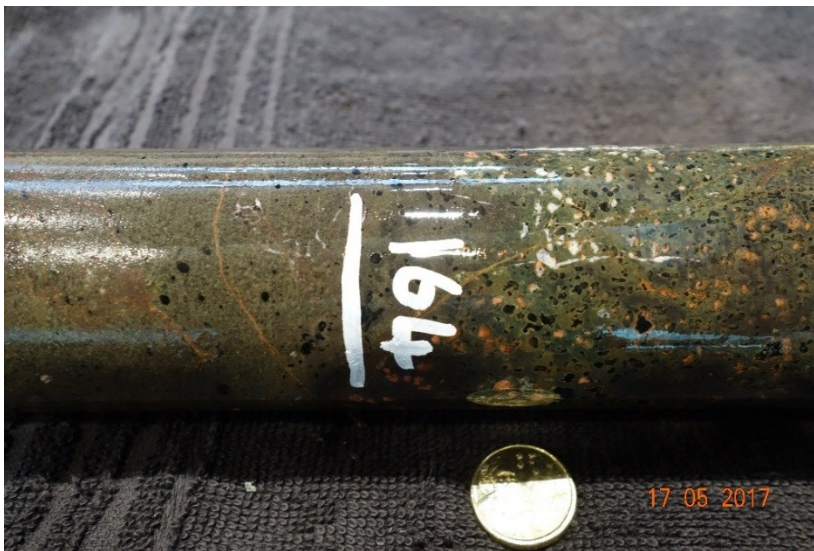
Figure 7. Core photograph showing abrupt juxtaposition of amygdaloidal and more dense basalt in the upper part of a flow unit at 164 m depth.
