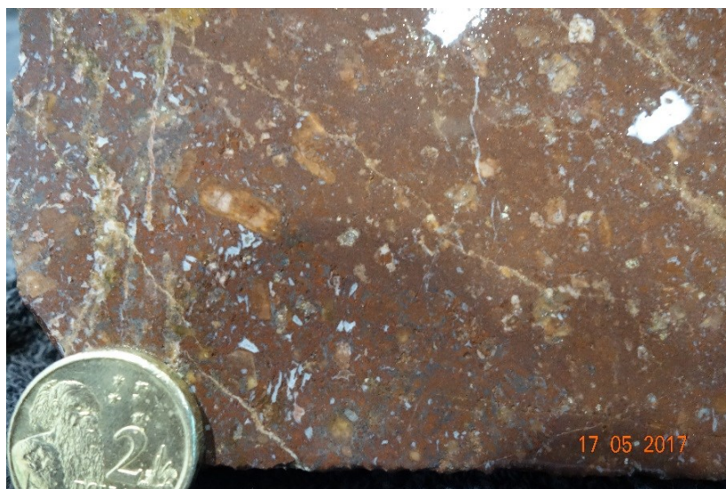
Core photo at 101.1 m (below) ; porphyritic texture and quartz amygdalae.
