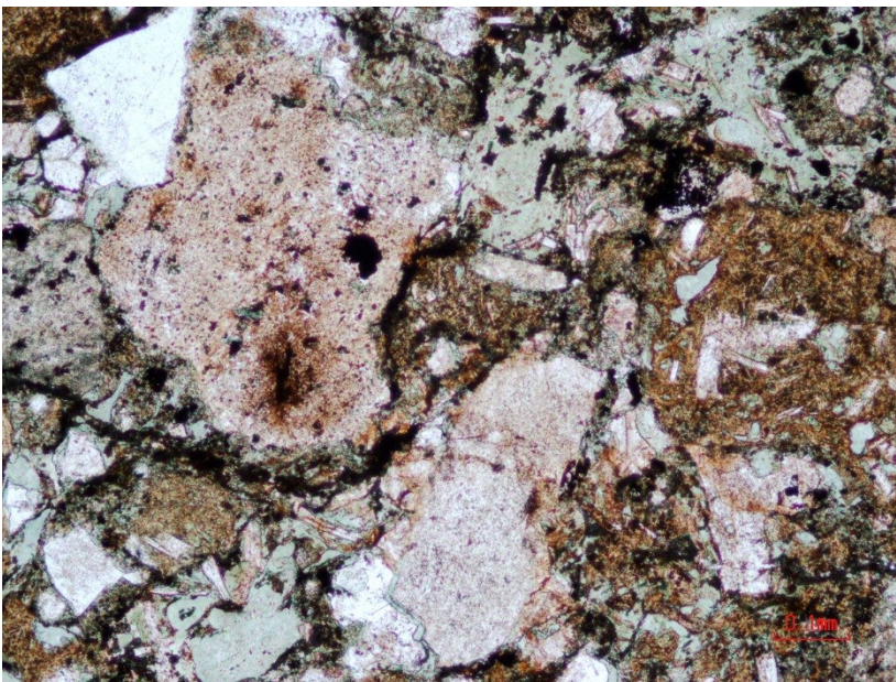
Figure 16. Photomicrograph in plane-polarised light highlighting some of the felsic volcanic component of the sandstone; quartz in upper left, pale pink micropoikilitic groundmass grain left of centre and pale alkali feldspar grain below centre. Most of the other grains in this view are of basaltic provenance including a fine brown basalt grain on right side and chlorite-replaced grains. From 260.92 m depth. X 10 lens, base of photo is 1.2 mm. (Sample 2332883).
