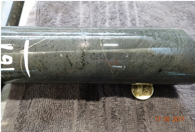
Figure 11. Core photograph of faint continuous flow foliation in the massive interior of basalt flow unit 3 at 166.9 m depth.
