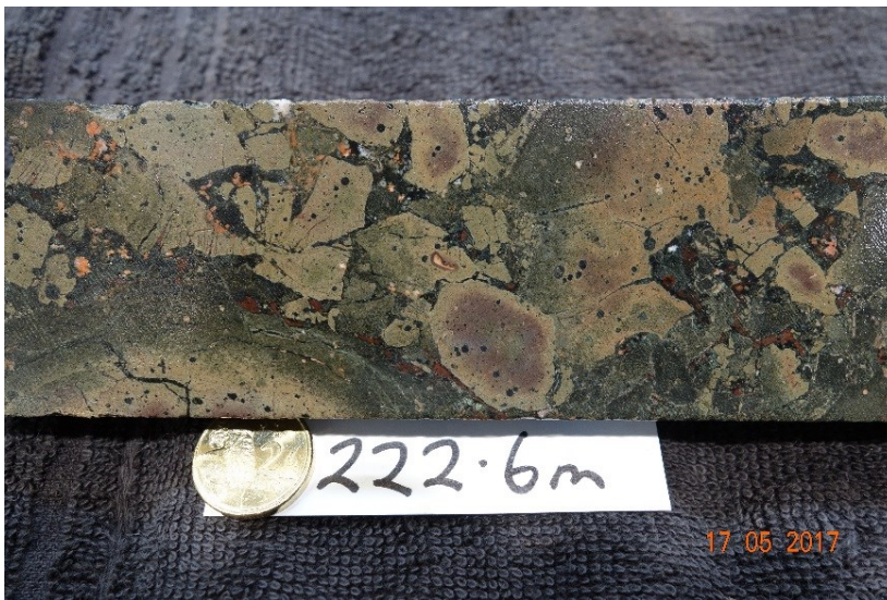
Figure 13. Core photograph of smoothly curved margin and rind of possible pillow and adjacent monomictic breccia (hyaloclastite) from 226.6 m depth.
