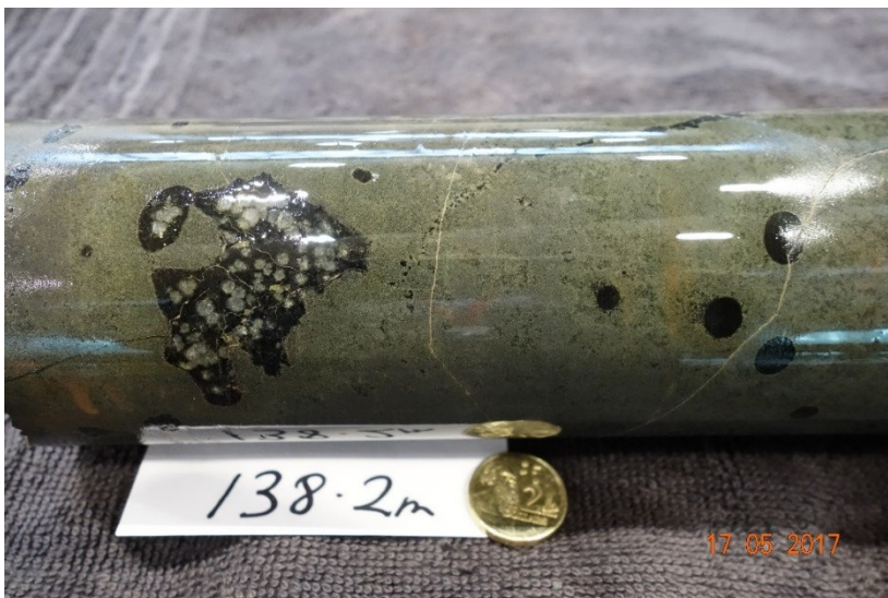
Figure 10. Core photograph of highly irregular and amygdaloidal clast within relatively dense basalt with scattered round chlorite amygdaloids at 138.2 m depth. The sample from the interior of a flow unit has a visibly coarser grained groundmass.
