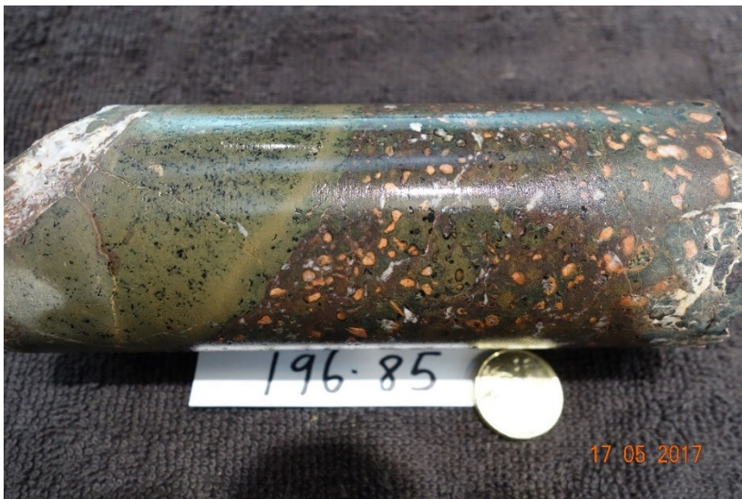
Figure 8. Core photograph of boundary between green, finely amygdaloidal basalt on left and more red/brown basalt with abundant and larger amygdales at 196.85 m depth; possible pillow margin.
