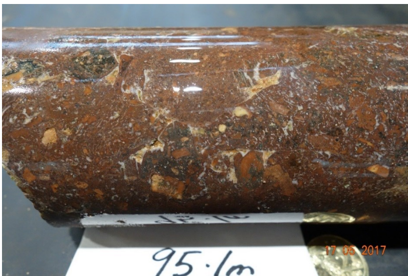
Figure 5. Core photograph showing brecciation in the lower part of the felsic volcanic unit (95.1 m depth) and the occurrence of small quartz-filled amygdales.
