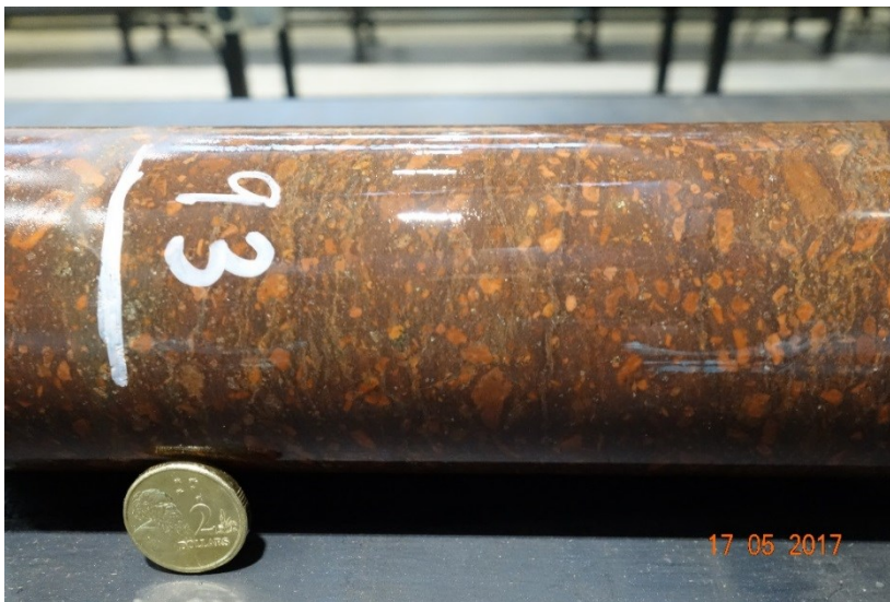
Figure 4. Core photograph showing flow foliation that is defined by paler folia in the groundmass and some alignment of plagioclase phenocrysts from 93 m depth.
