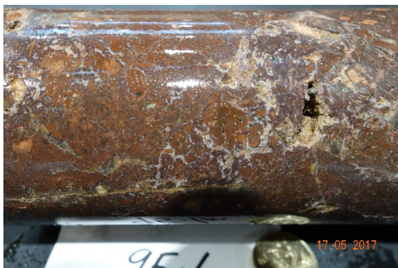
Small irregular quartz-filled amygdalae visible, slightly vuggy.
