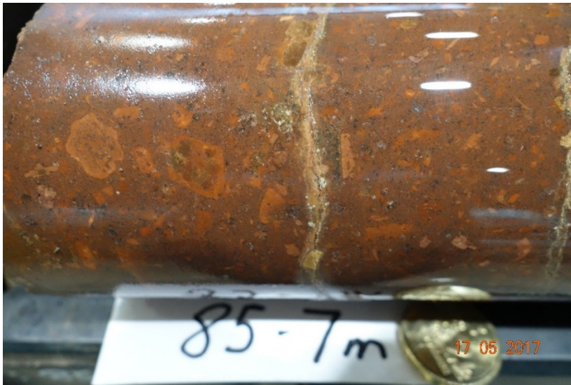
Figure 2. Core photograph showing the evenly porphyritic texture (mostly plagioclase and minor small altered ferromagnesian minerals) of the felsic volcanic unit from 85.7 m depth.
