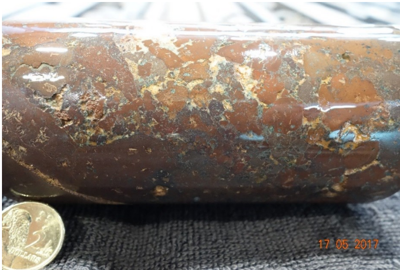
Figure 9. Core photograph of hematite-altered breccia; possible autobrecciated upper part of basalt flow unit at 104.95 m depth.
