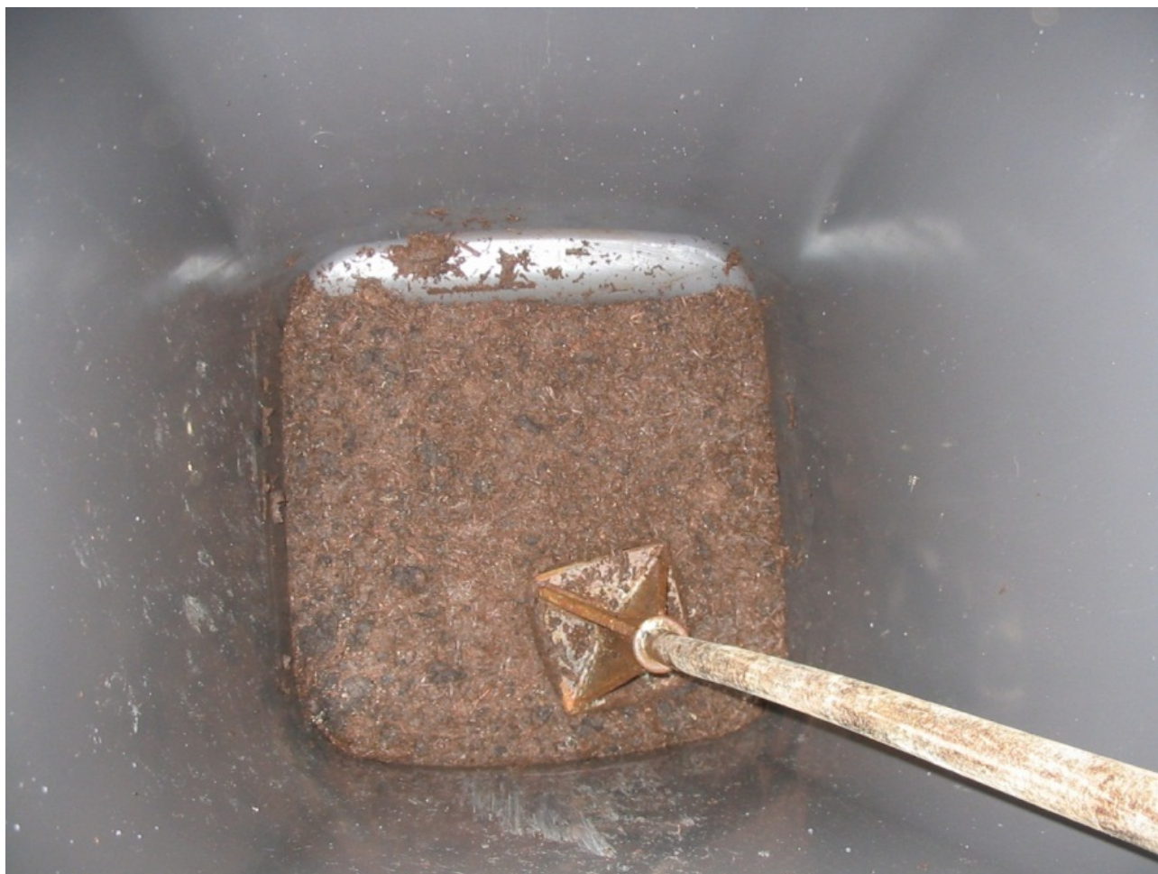
Figure 10. Compacting organic material in large-scale column. (Photo 414511)
