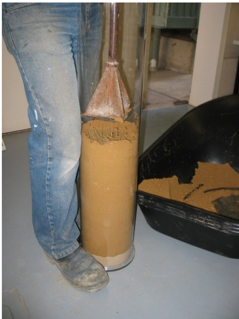
Figure 6. Loading column and compacting solid material. (Photo 414507)
