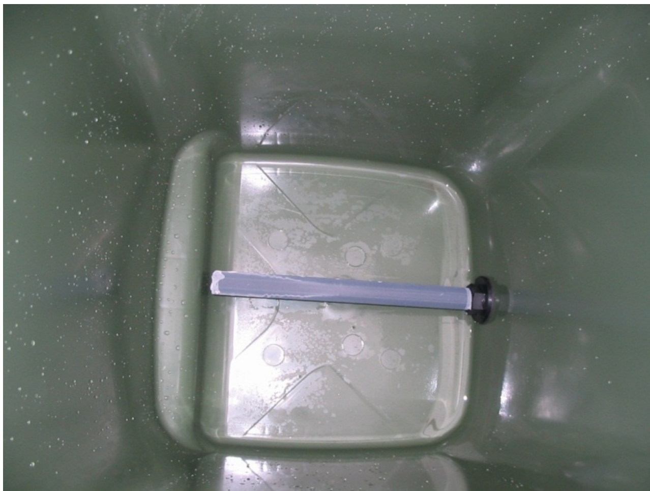
Figure 8. Drainage pipe in large-scale column, wrapped in 100 µm filter mesh. (Photo 414509)
