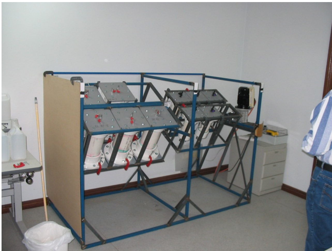
Figure 4. Bottle-roll leach testwork carried out at On Site Technology Pty Ltd. (Photo 414505)
