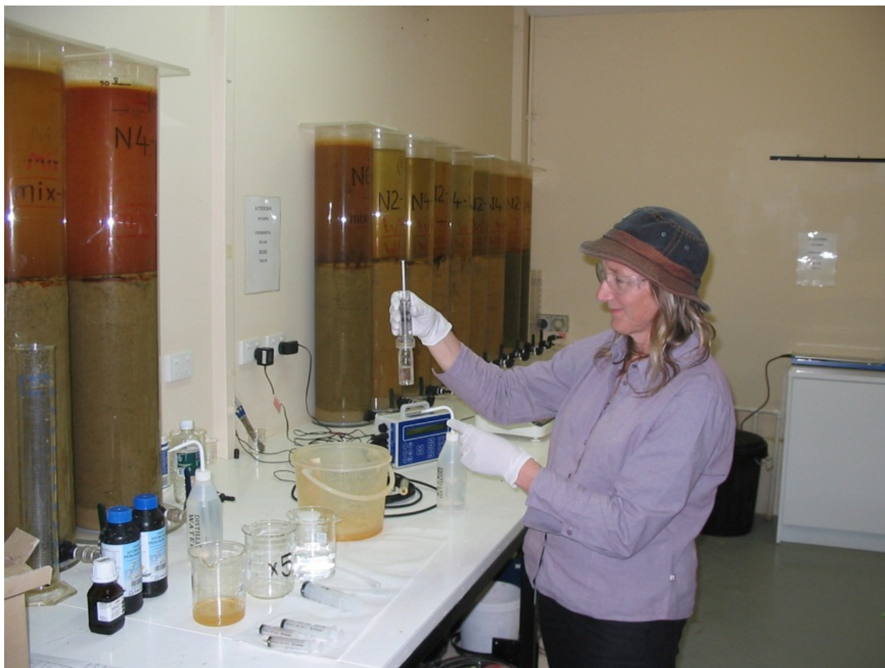
Figure 17. Testing leachate acidity in the Brukunga lab using an Earth Systems micro-titrator. (Photo 414518)
