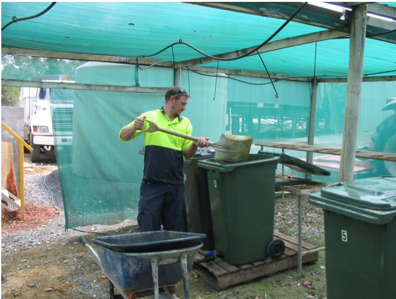
Figure 9. Loading PAF material into a large-scale column (plastic bin). (Photo 414510)
