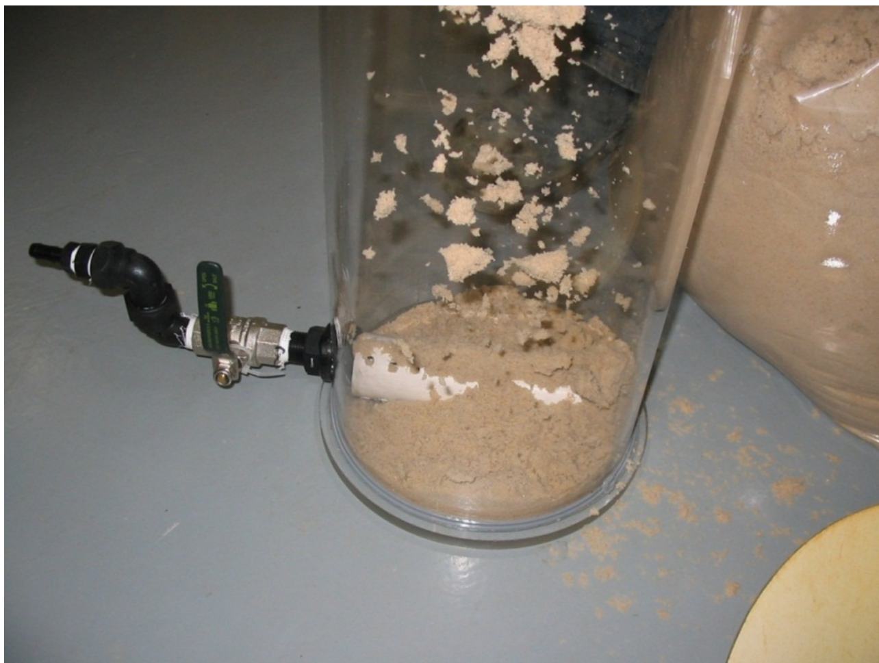
Figure 5. Adding a filter layer of sand at base of new column. (Photo 414506)
