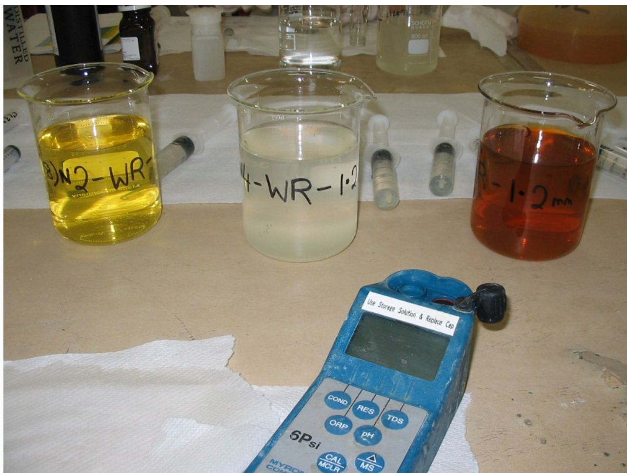
Figure 16. Testing leachate samples with the Myron ultrameter. (Photo 414517)
