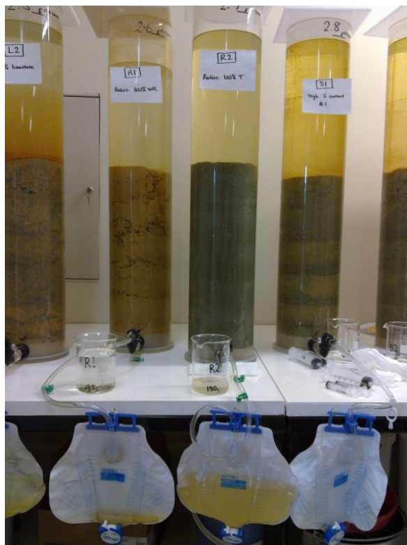
Figure 7. Collecting leachate from stage I columns into drainage bags.
