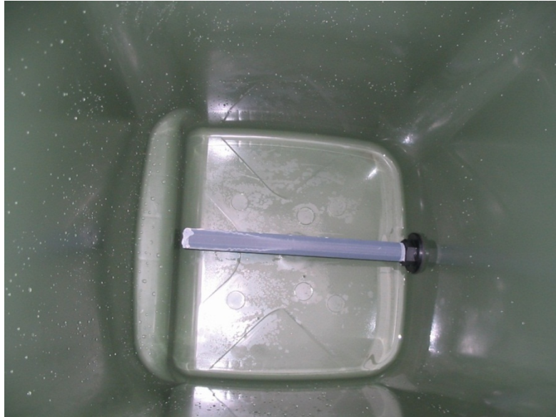
Figure 8. Drainage pipe in large-scale column, wrapped in 100µm filter mesh.
