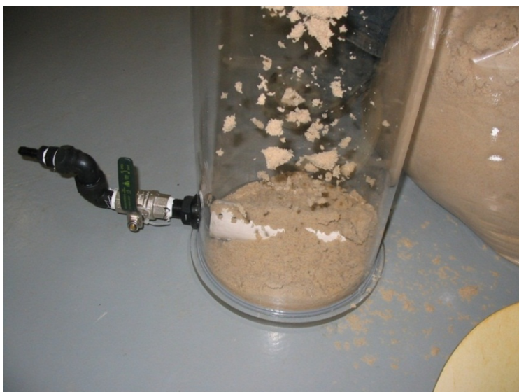
Figure 5. Adding a filter layer of sand at base of new column.
