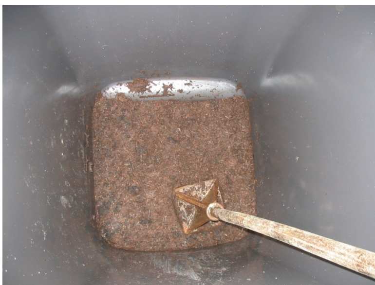
Figure 10. Compacting organic material in large-scale column.
