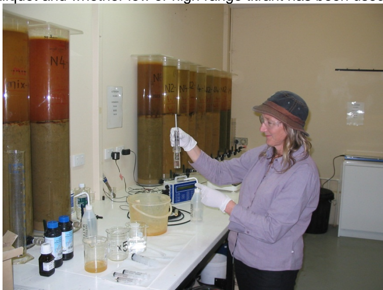
Figure 17. Testing leachate acidity in the Brukunga lab using an Earth Systems micro-titrator.
