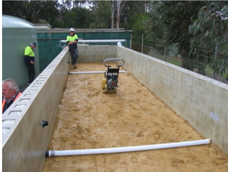
Figure 14. Piezometers placed horizontally across the width of the test-cell.
