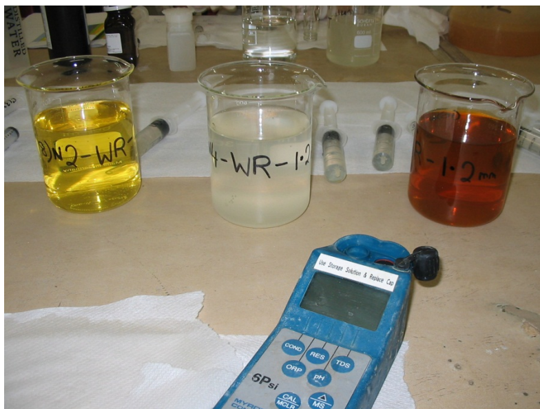
Figure 16. Testing leachate samples with the Myron ultrameter.
