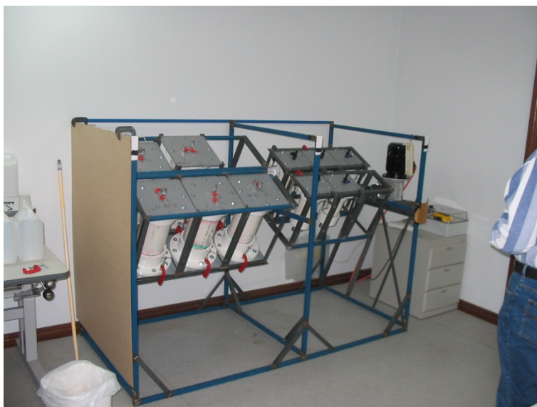
Figure 4. Bottle roll leach testwork carried out at On Site Technology Pty Ltd.
