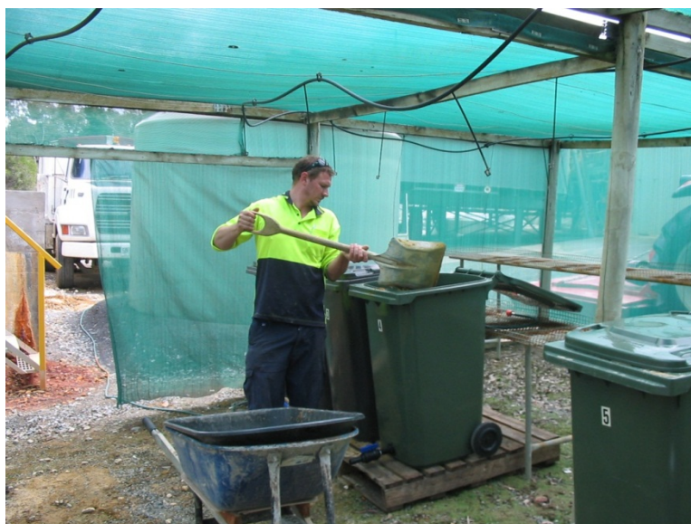
Figure 9. Loading PAF material into a large-scale column (plastic bin).
