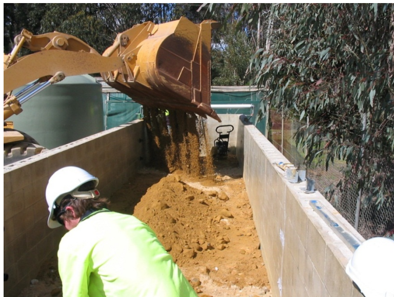
Figure 12. Dumping PAF mix into the geochemical test-shell, composed of besser blocks.
