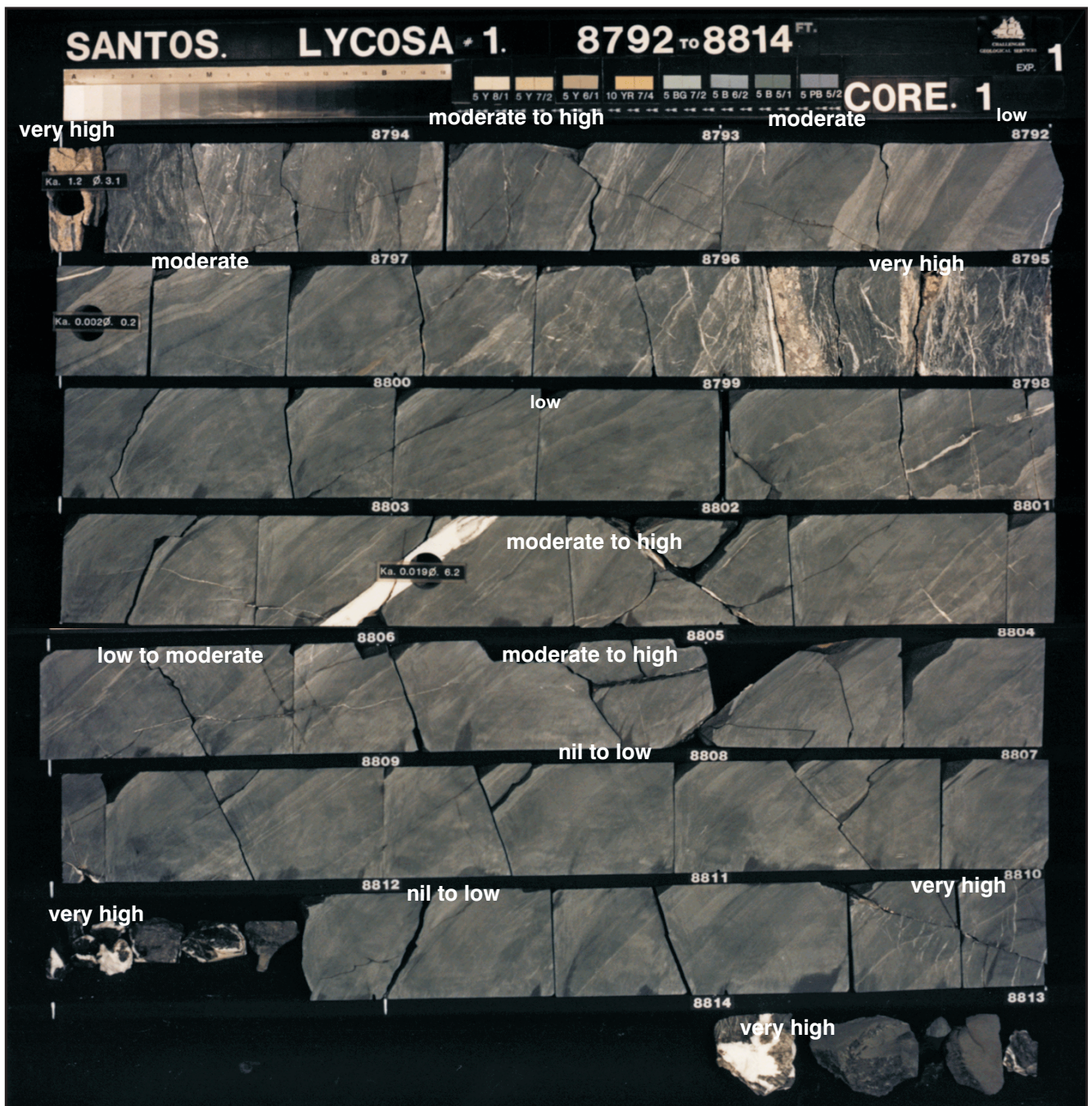
Fig. 13 Core 1, Lycosa 1, 8792-8814', showing main fractures on slab surface; fracture density is not even, and varies from low over the intervals 8799-8801' and 8807-8809'10", high to very high over the interval 8794-8797'. Density variations are marked to the left of the core intervals.
