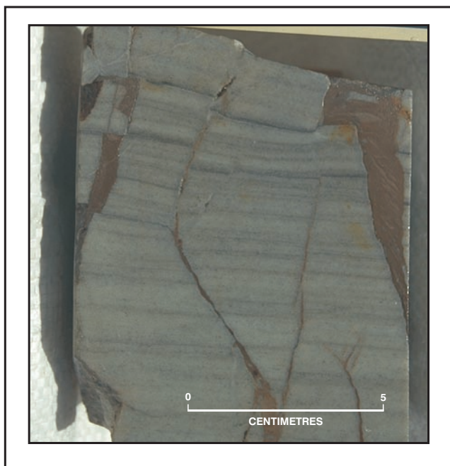
Fig. 8 Vuggy fractures in Coonatie 1, core slab, 10400'6". (Photo 046713)
