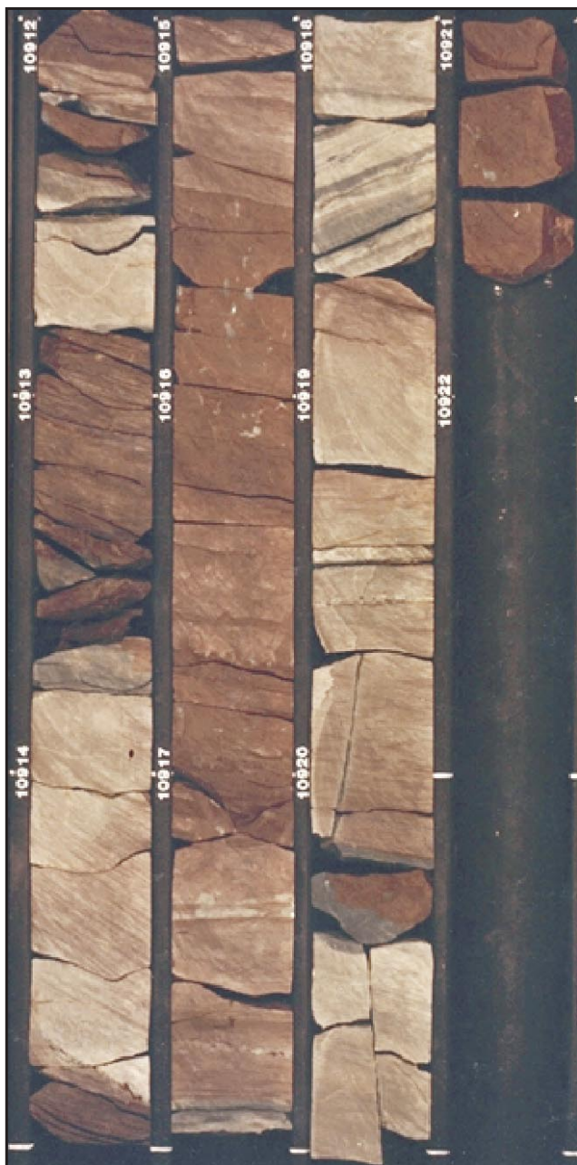
Fig. 34 Core photo in Meranji 2, showing low grade of fracture density.
