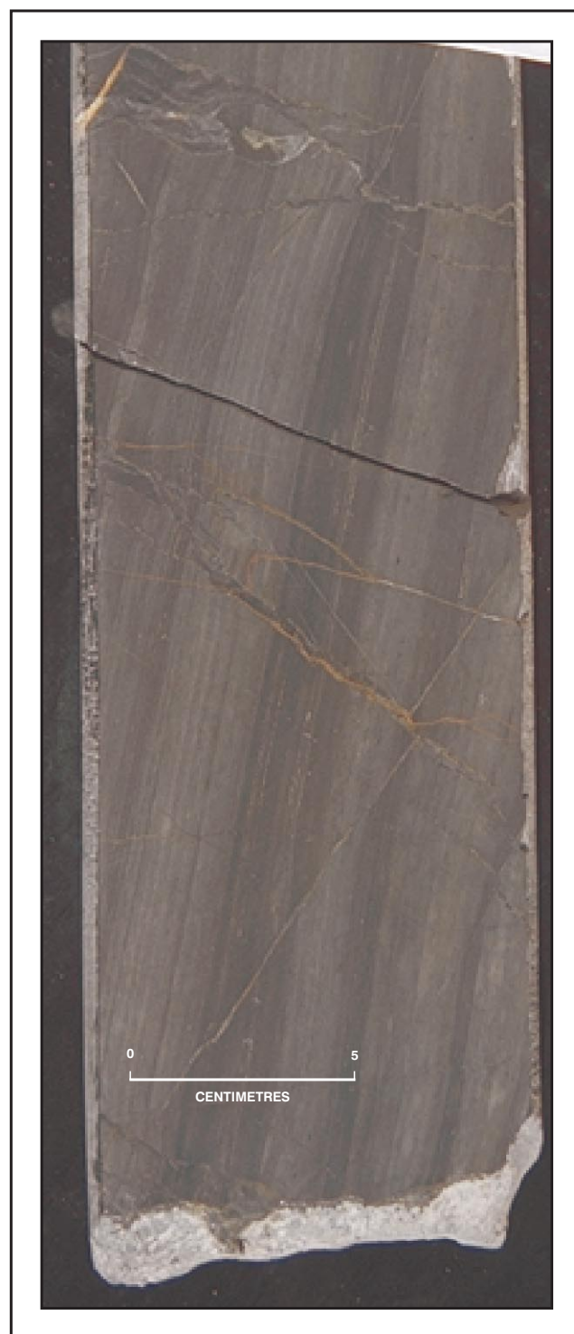
Fig. 21 Mudlalee 1 core, illustration of fracture sets. (Photo 046741)
