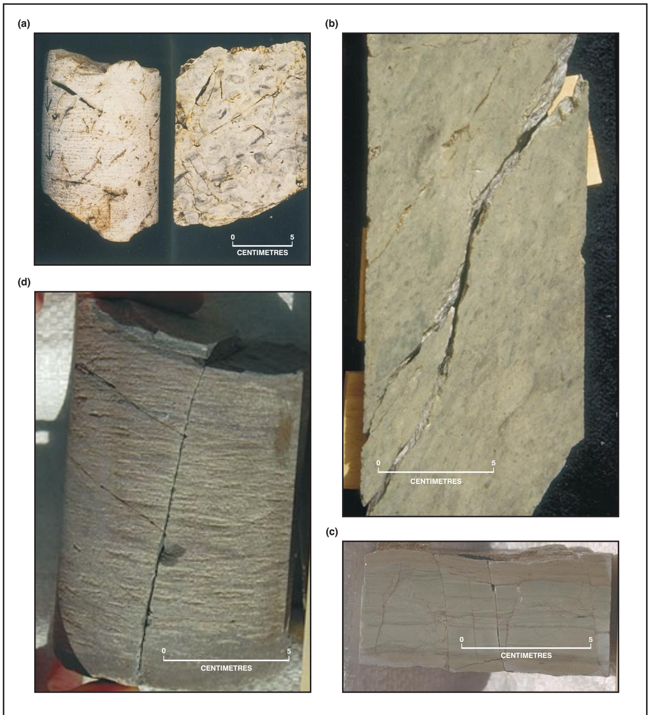
Fig. 5 (a) Core photo, showing open fractures connecting vuggy porosity in dolomite, Gidgealpa 5, 8118'. (b) Open fracture in ignimbrite from Boxwood 1, 6154.5'. (c) Core photo, showing open fracture and other filled fractures along normal microfaults, Gidgealpa 4, 7226'8-9". (d) Open fracture in core, Meranji 2, 10920'. (Photo 046698, 046699, 046700 and 046701).
