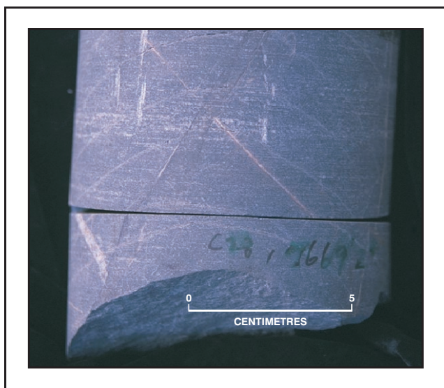
Fig. 3 Petal fractures (induced) in sandstone from Dullingari 1, core 28, at 9669'2". (Photo 046695)
