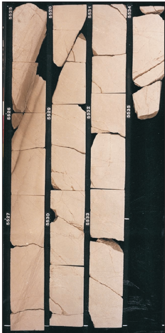
Fig. 31 Core photo in Jennet 1, showing possible open fractures in brittle coarse sandstone.
