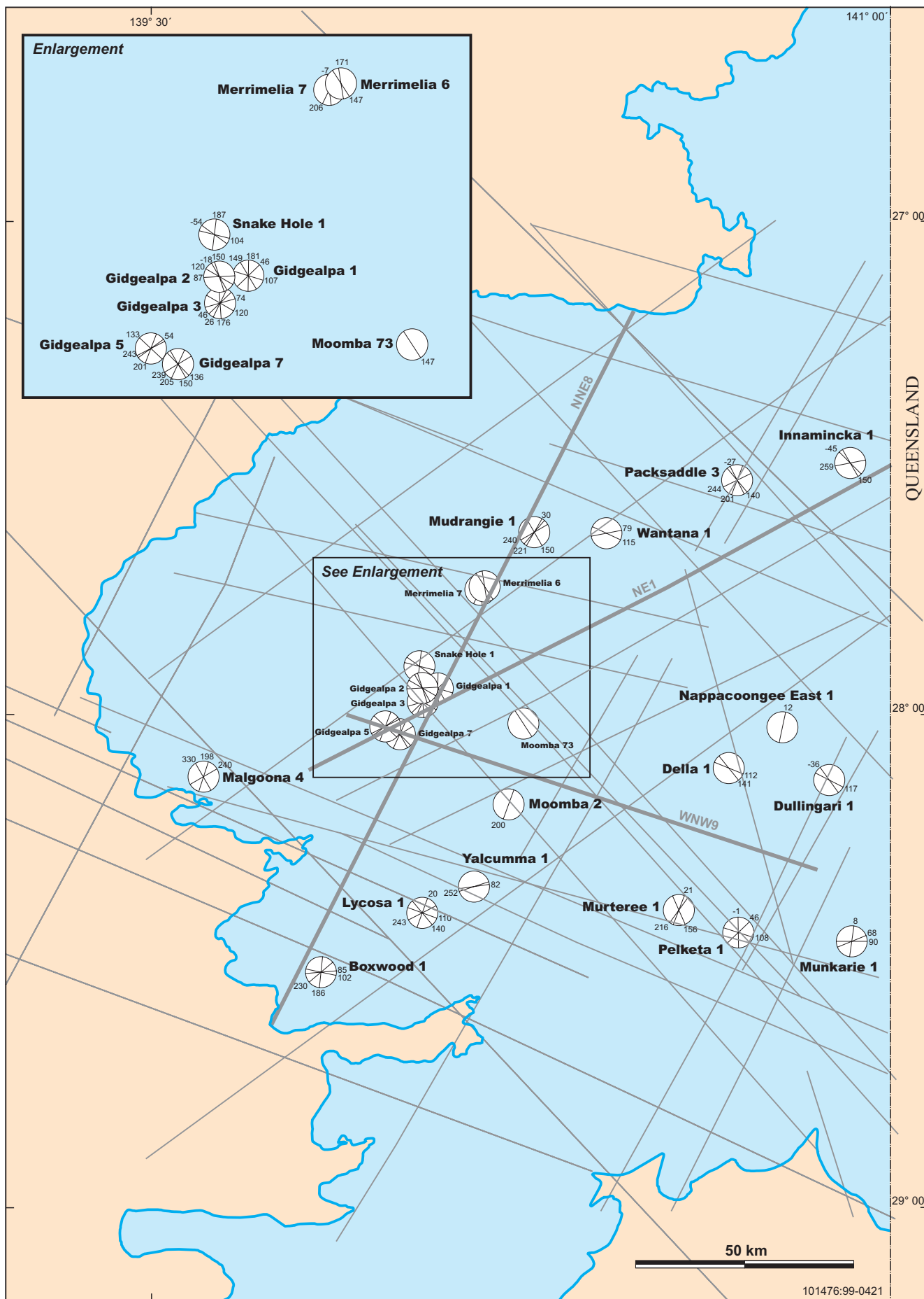
Fig. 30 Map of Cooper Basin showing absolute strike orientations of steep fractures (circled) to low frequency lineaments (LFL), NNE8, WNW9 and NE1 identified by Boucher (1998).
