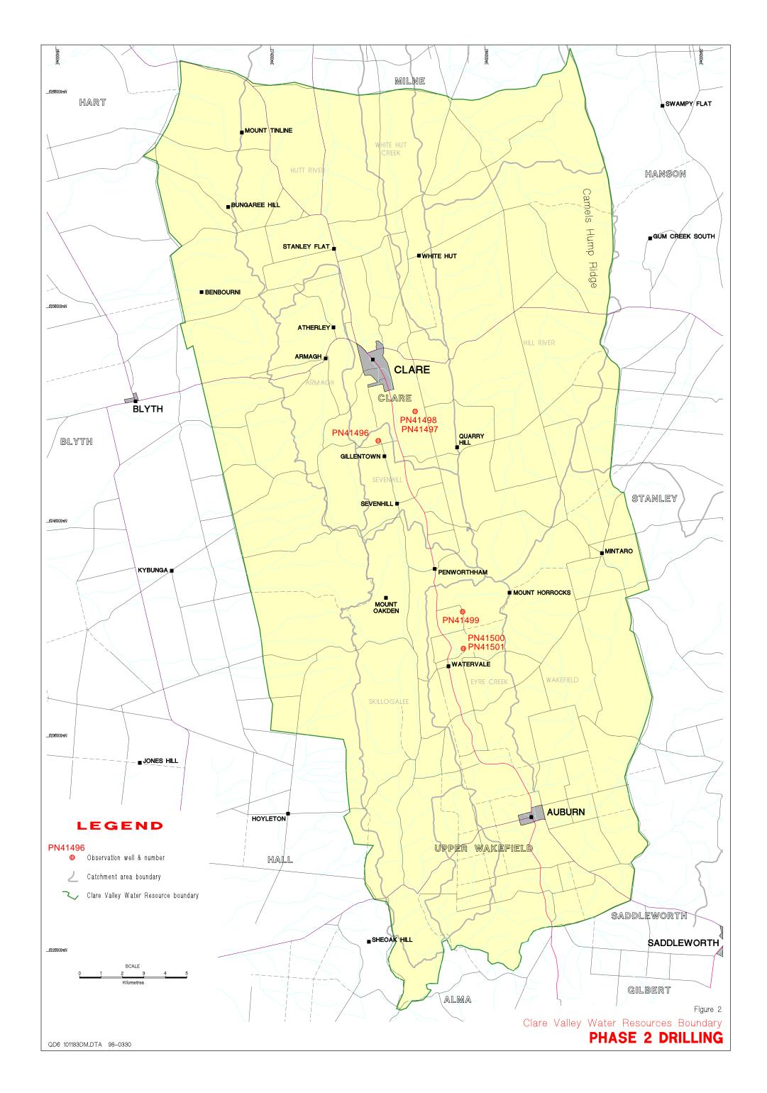
A tabulated summary of Phase II drilling is presented in Appendix A and geological logs are contained in Appendix B. All bores drilled were completed open hole with surface casing installed into the soft sediment until hard rock was encountered, generally at a depth between 4 to 9 meters. The aim of the phase II drilling exercise was to provide additional bores to further enhance investigations into the hard rock aquifer properties of Clare (an ongoing joint venture between PIRSA and CSIRO).
