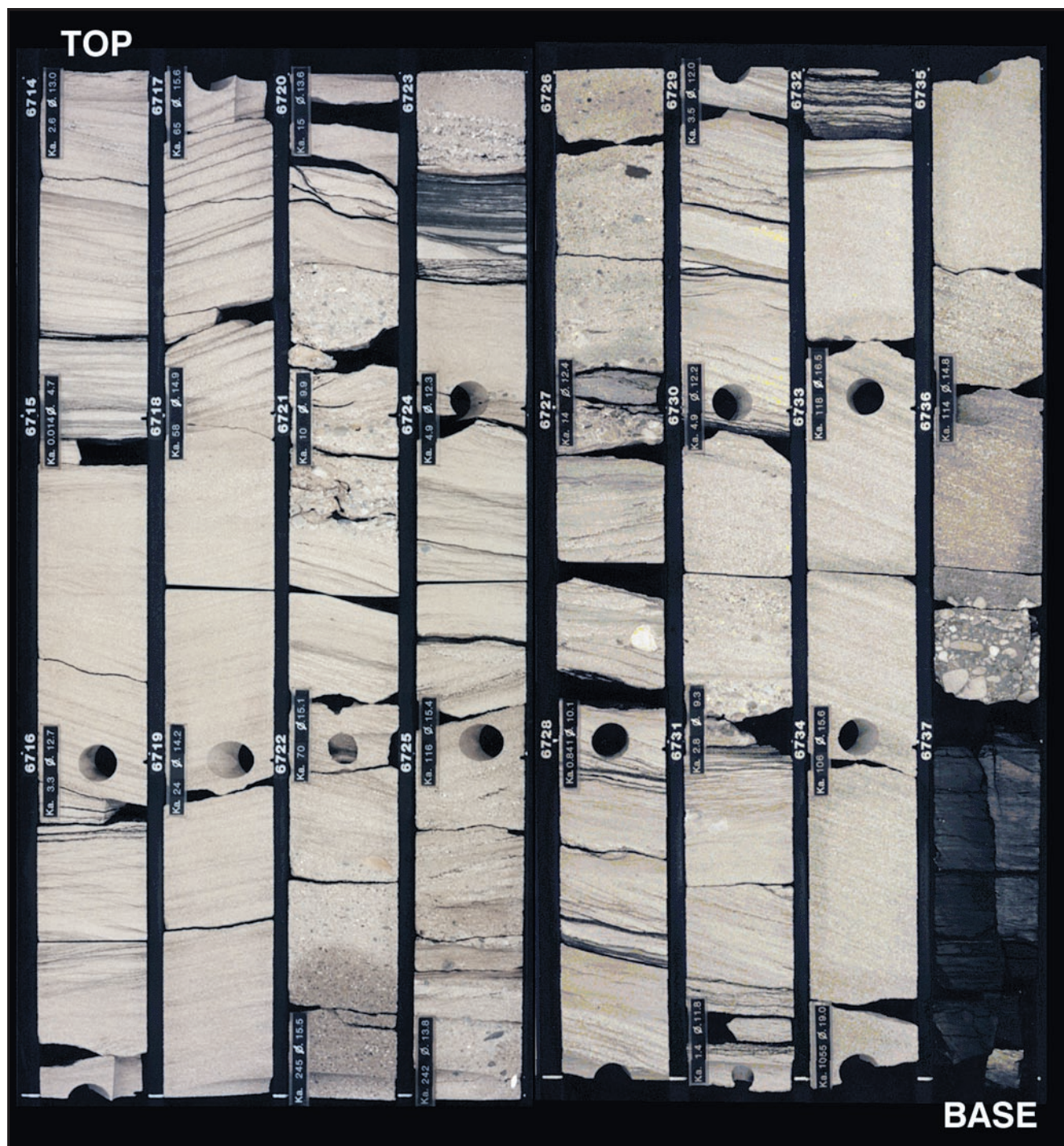
Compound bar form with internal scours and basal lags in the Patchawarra Formation, Kujani 2, 2046–2054 m. (Photo 46500)
