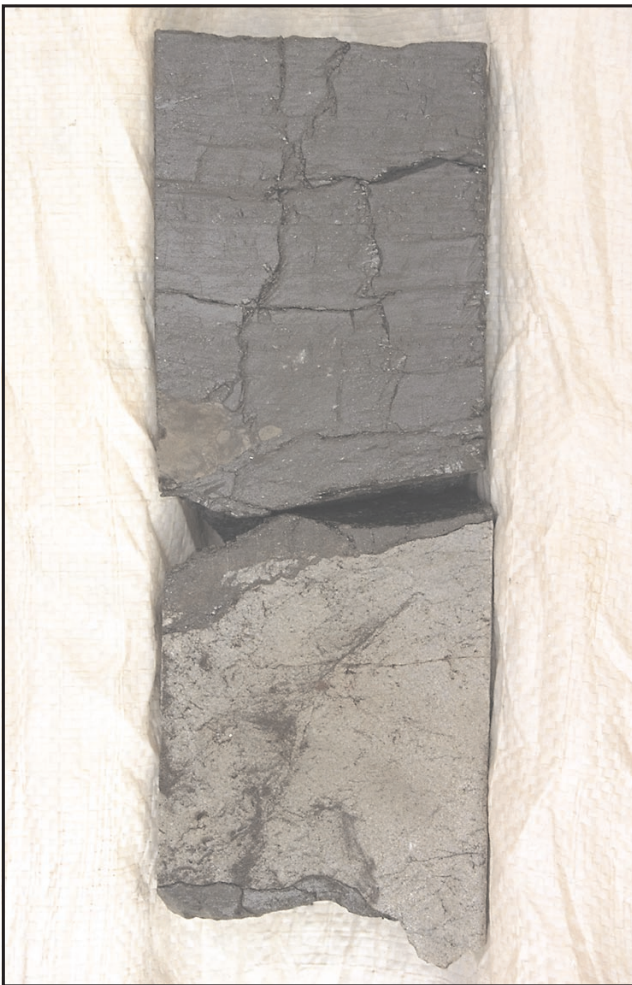
Porous, permeable sandstone overlain by coal with no intervening shale in the Epsilon Formation, Cuttahirrie 3, core 1, 2902.3 m (driller). Fractures in coal induced by unloading. Core diameter 100 mm. (Photo 46326)
