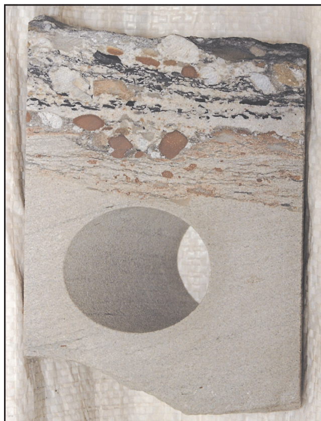
Disconformable contact between Jurassic Hutton Sandstone and Triassic Arrabury Formation, Marabooka 3, core 1, 1865.3 m (driller). Fine-grained Arrabury Sandstone has porosity 8.5% and permeability 0.17 mD. Core diameter 100 mm. (Photo 46051)
