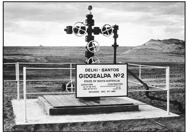
Gidgealpa 2 capped by a 'Christmas tree' and ready for gas production. (Photo N013046)
