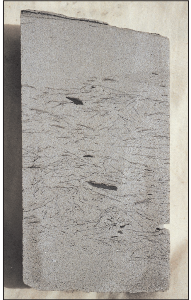
Carbonaceous fragments in a fine to medium-grained sandstone in the Patchawarra Formation, Fly Lake 4, 2709 m. (Photo 45940)
