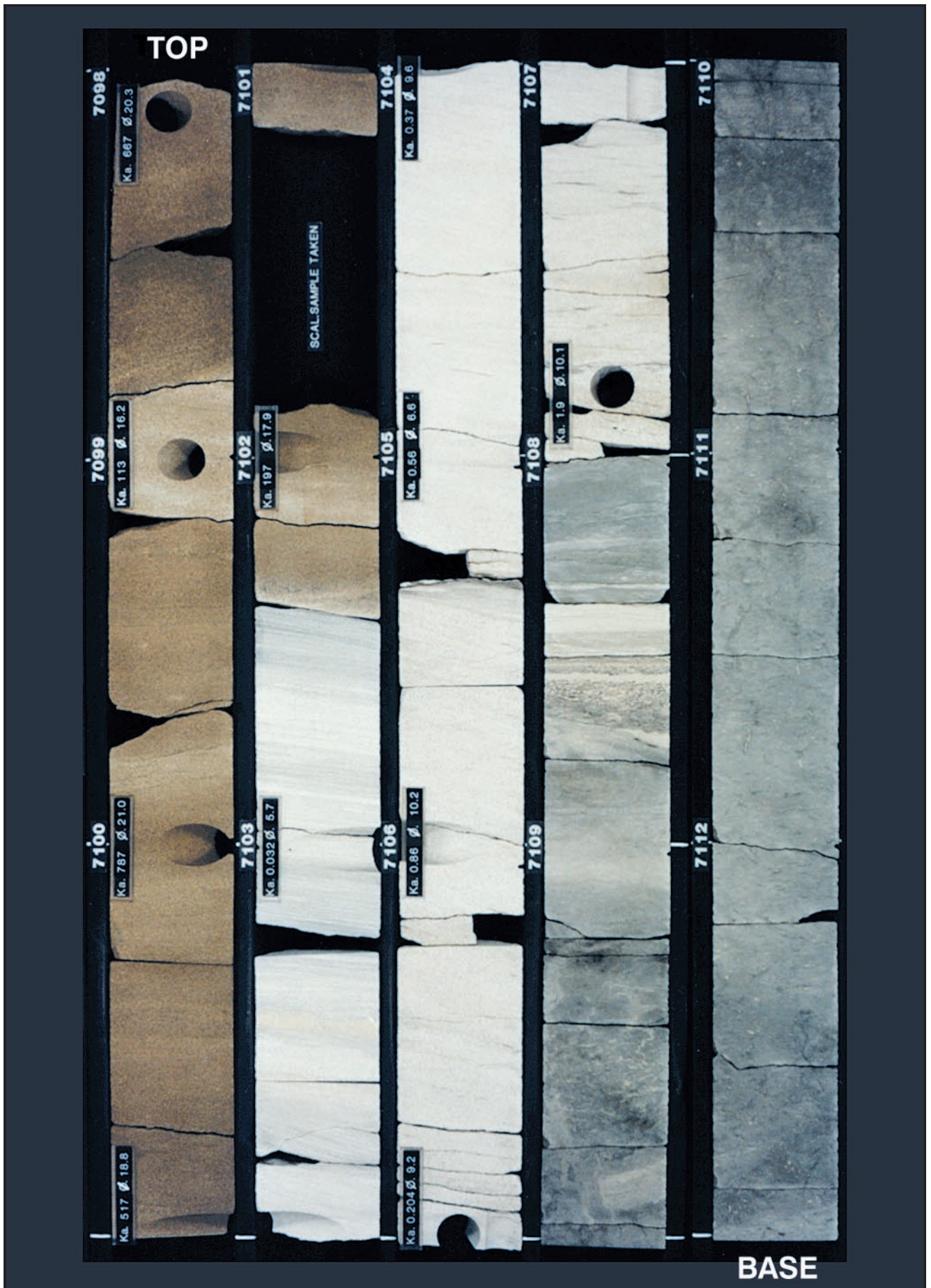
Callamurra and Paning Members, Merrimelia 29, 2164–2168 m. The upper Callamurra Member consists of a palaeosol developed in a silty mudstone. This is overlain sharply by Paning Member channel sandstone. (Photo 46503)
