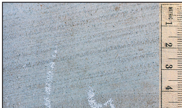
Wind ripple laminations ('pinstripes') on aeolian dune in the Merrimelia Formation, Merrimelia 5, 2624 m. (Photo 46497)
