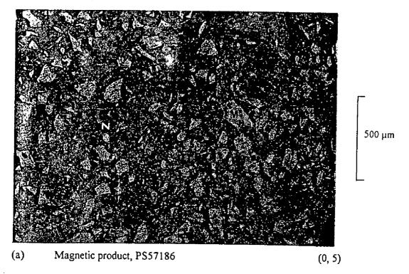
This sample consists mainly of magnetite (M) with smaller amounts of non-opaque gangue (N). The labelled non-opaque gangue particle is locked with magnetite.
