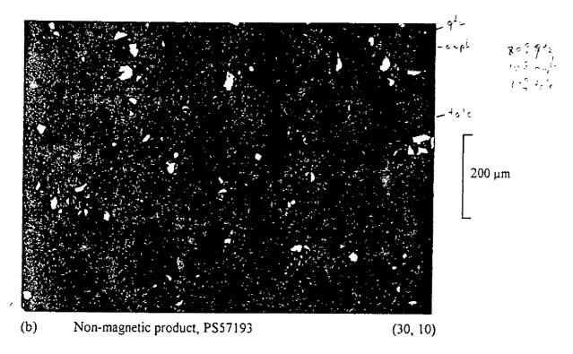
This sample consists mainly of non-opaque gangue with minor magnetite.
