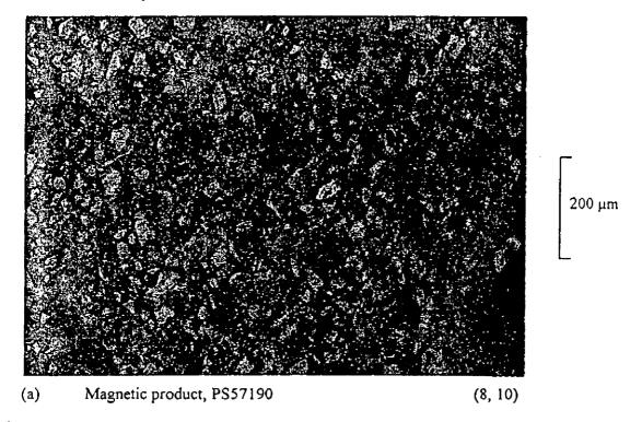
This sample consists mainly of magnetite with minor non-opaque gangue. A hematite particle (bluish-grey) is located near the centre of field.
