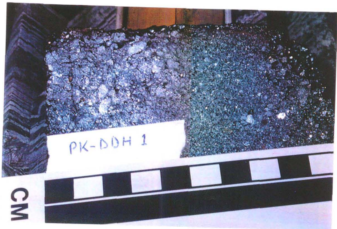
Photo 6 Peculiar Knob Deposit, coarse grained massive specular hematite (Photo No. 44369).
