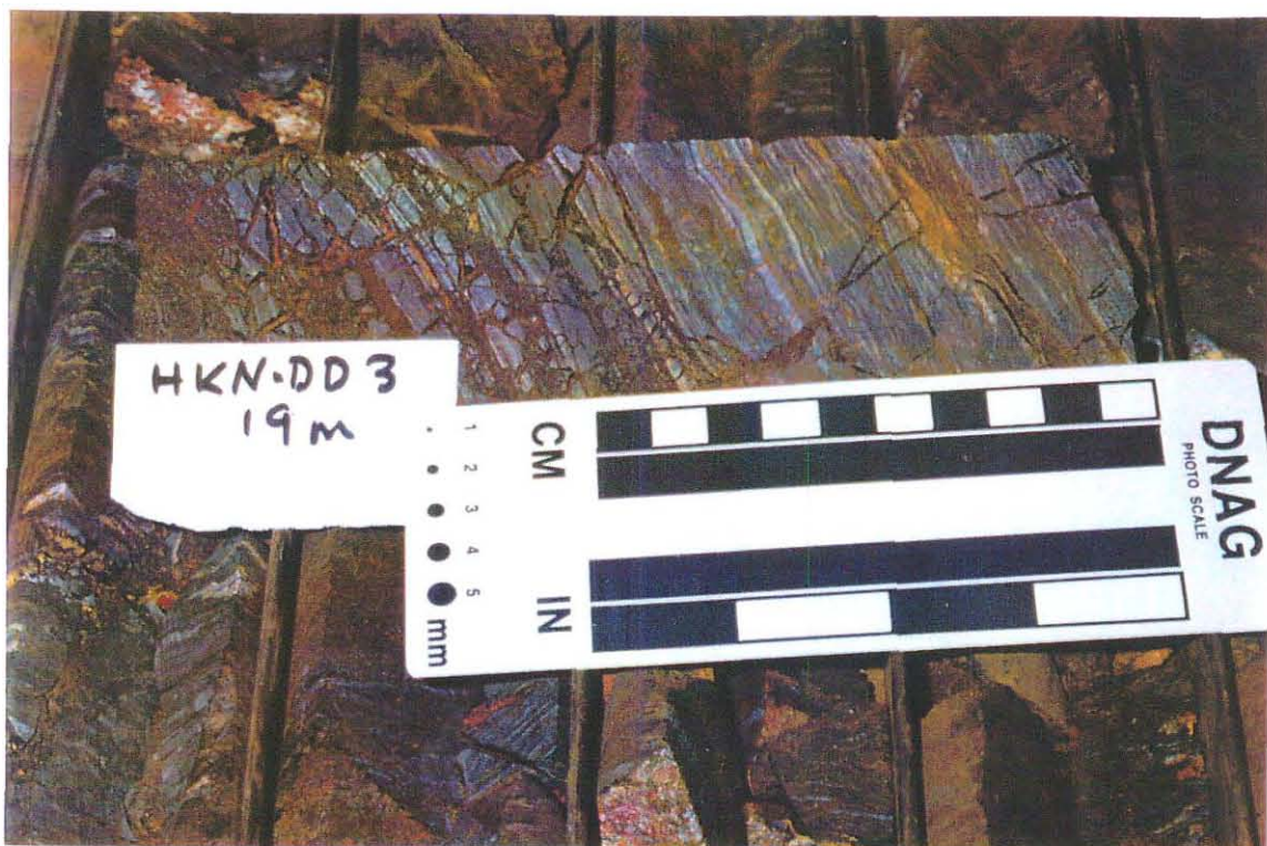
Photo 4 Kestrel Deposit, supergene oxidised BHIF (Photo No. 443670).
