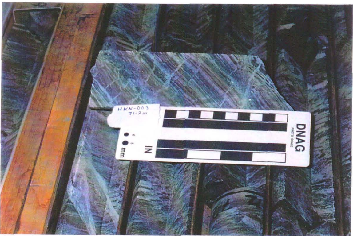
Photo 1 Kestrel Deposit, thinly laminated BIF with micro faulting and amphibole veinlets (Photo No. 44364).
