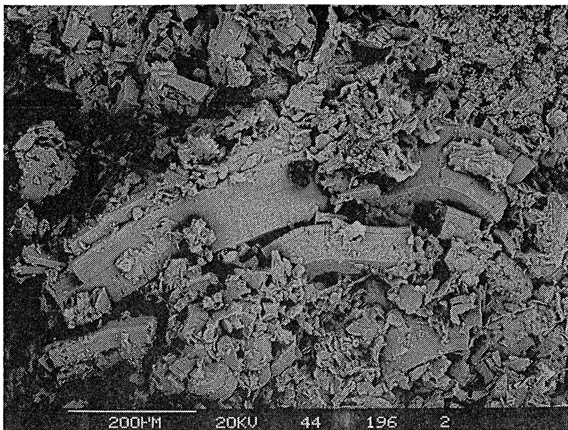
Plate 6. Tomney West. TW2. Sample SB050. Coarse vermicular kaolinite within a matrix of stumpy kaolinite books and coarse kaolinite plates. Halloysite present on surface of coarse kaolinite books. Bar scale 200µm, photo. no. 44/196.
