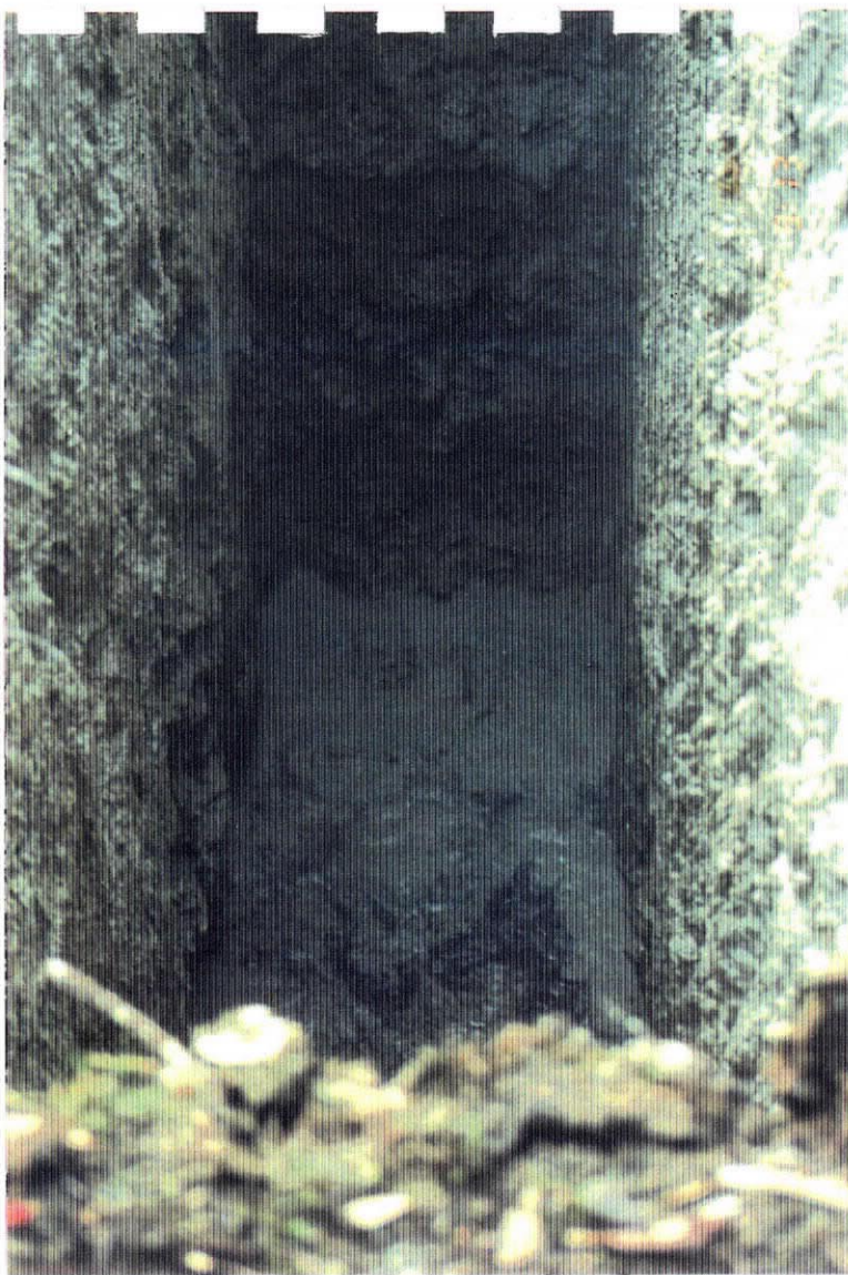
PLATE 3: Pit 9 - Note stable, smooth walls; recovering groundwater level. Photo No. 40285
