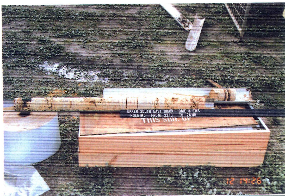
PLATE 25: SITE 2, Borehole M5. Core sample from 23.10 m to 24.40 m depth Photo No 40307
