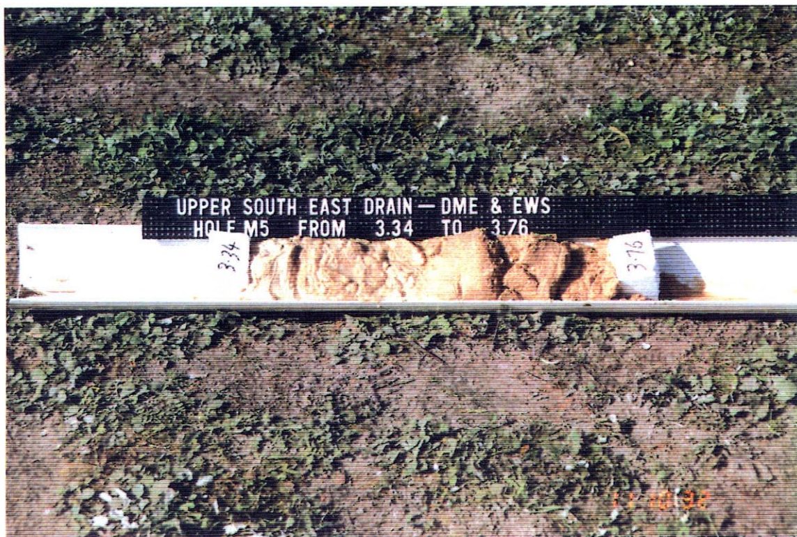
PLATE 22: SITE 2, Borehole M5. Core sample from 3.34 m to 3.76 m depth Photo No 40304
