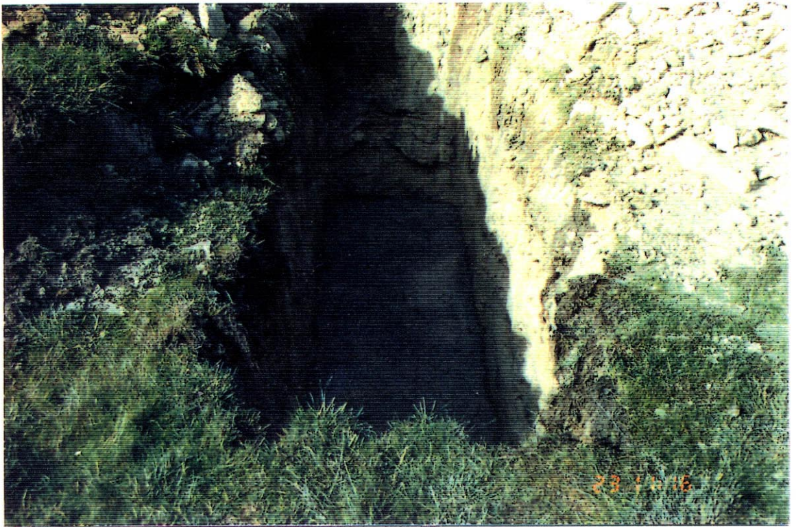
PLATE 1: Pit 7 - Note stable walls and groundwater recovered almost to Standing Water Level (SWL). Photo No. 40283
