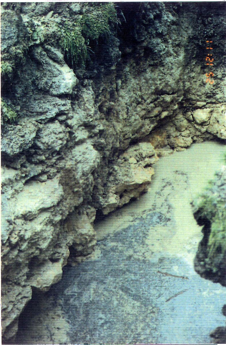
PLATE 10: Pit 13 Note rough, ragged walls, high SWL. Photo No. 40292
