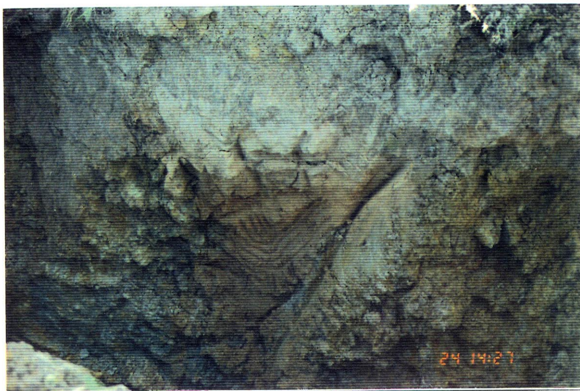
PLATE 7: Pit 11 - Note stable pit wall, "sand dyke" extending down into calcrete/clay mixture.
