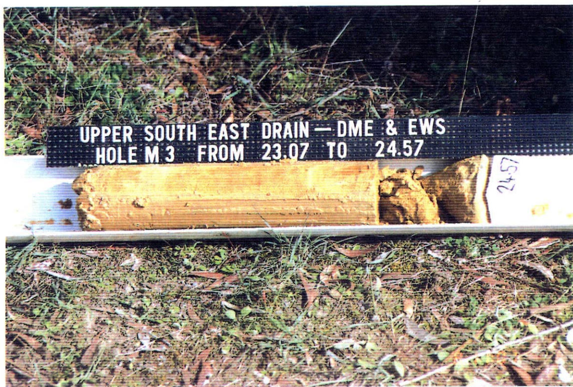
PLATE 20: SITE 1, Borehole M3. Core sample from 23.07 m to 24.57 m depth Photo No 40302
