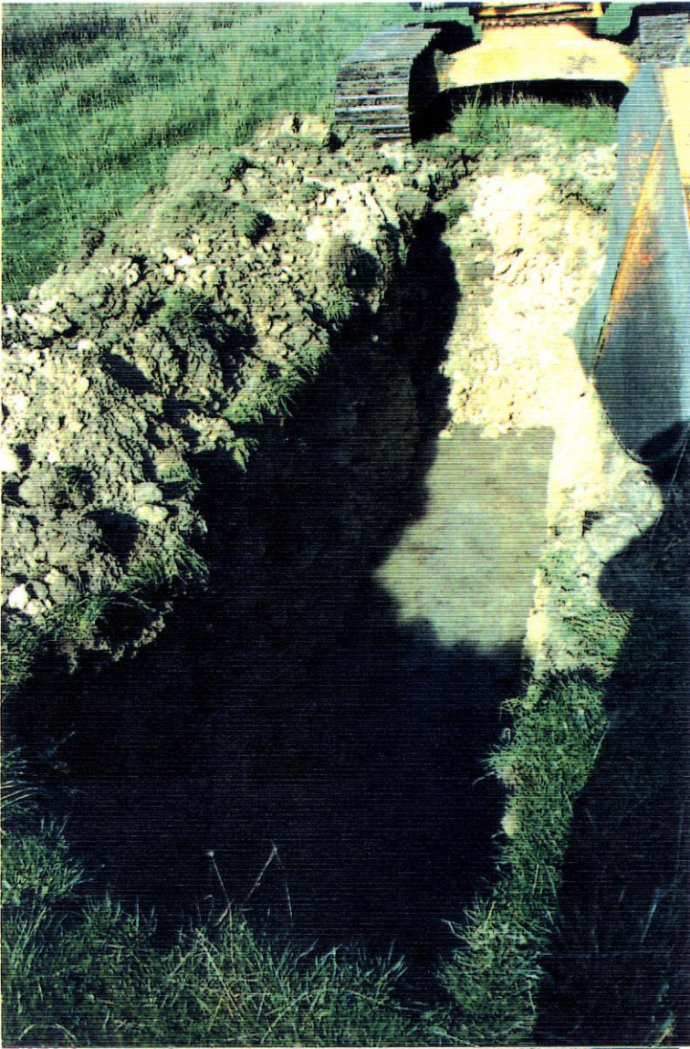
PLATE 5: Pit 10 - Note stable walls, high SWL after rapid recovery. Photo No. 40287
