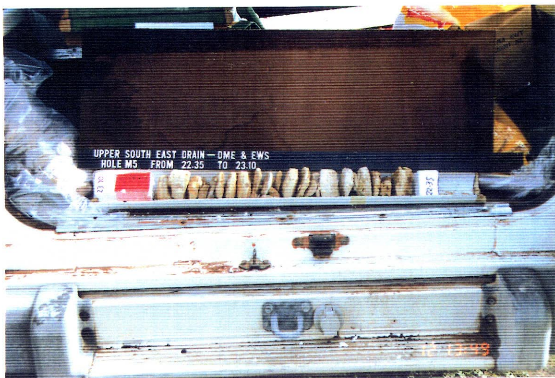
PLATE 24: SITE 2, Borehole M5. Core sample from 22.35 m to 23.10 m depth Photo No 40306
