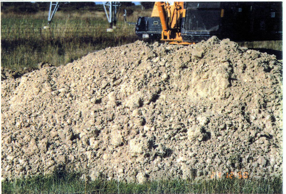
PLATE 6: Pit 10 - spoil - note nodular/blocky nature of calcrete spoil. Photo No. 40288
