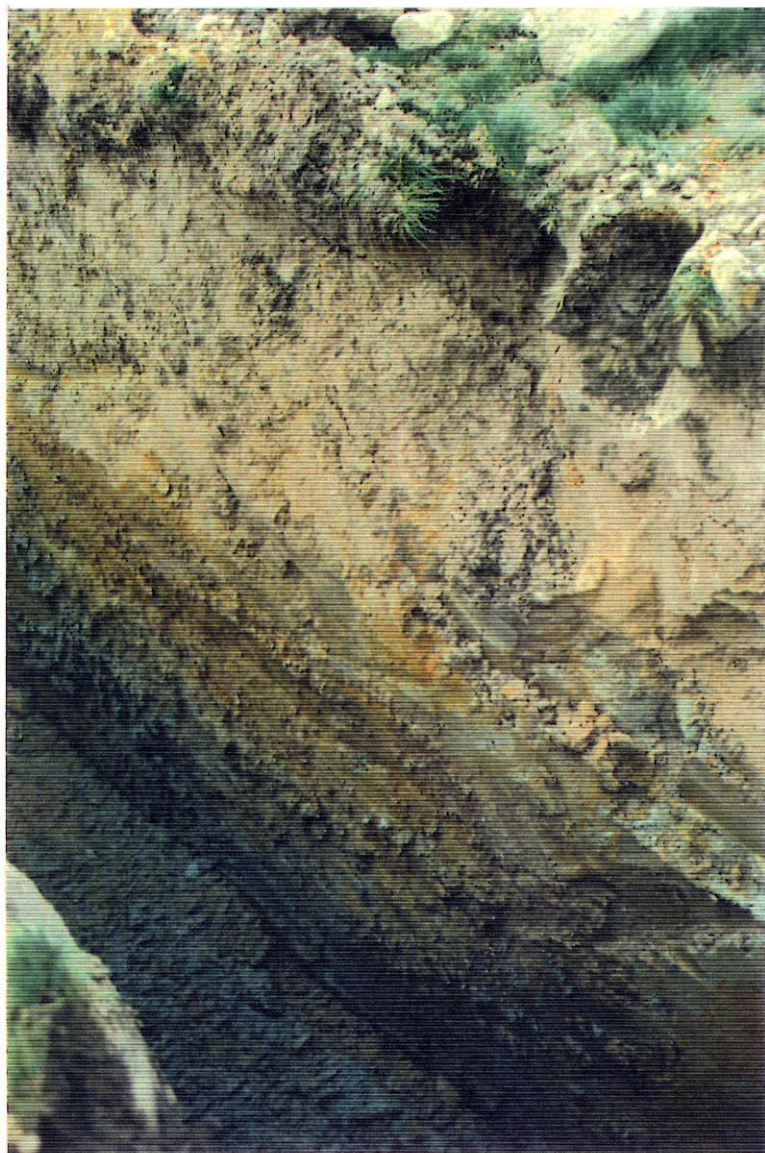
PLATE 9: Pit 12 - Note smooth clayey wall of top section, tight nature of clays (below SWL - but little seepage). Photo No. 40291
