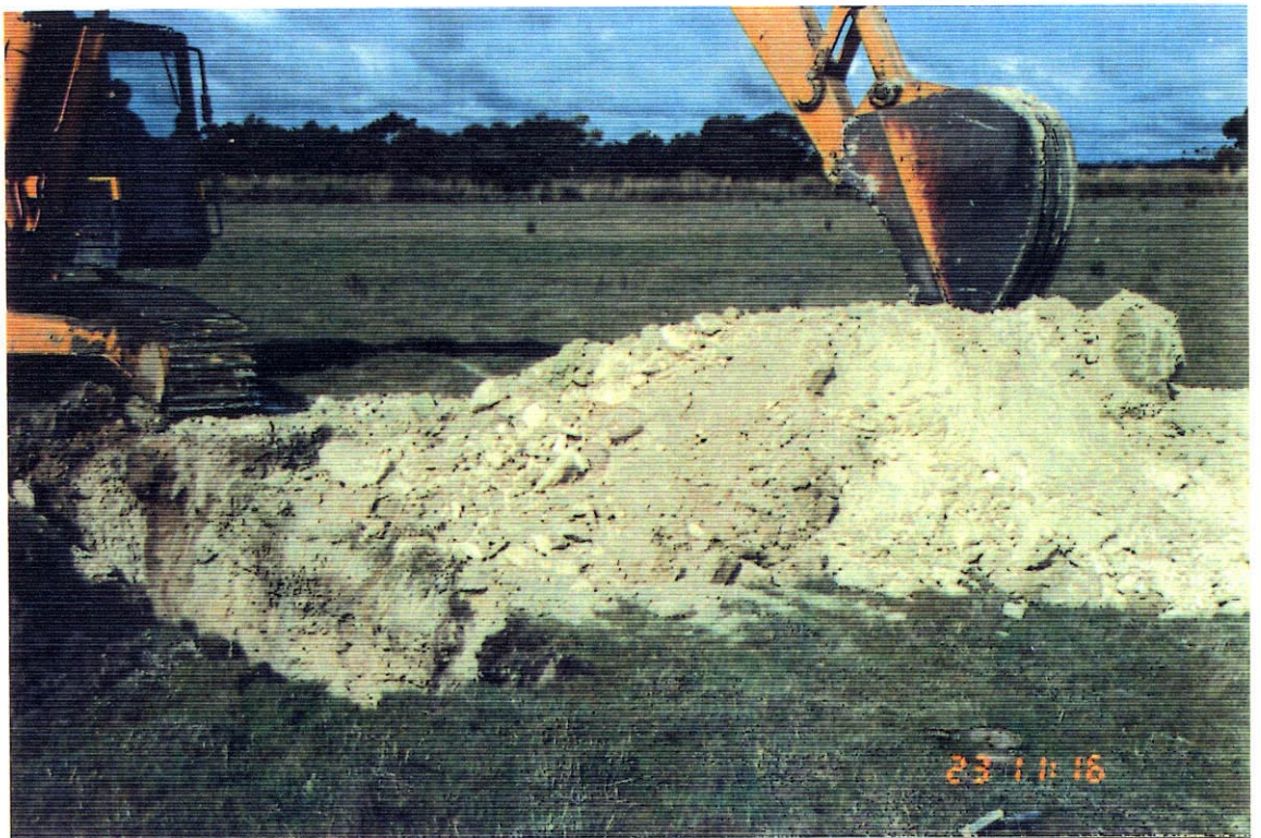
PLATE 2: Pit 7 - spoil - note granular and blocky nature. Photo No. 40284
