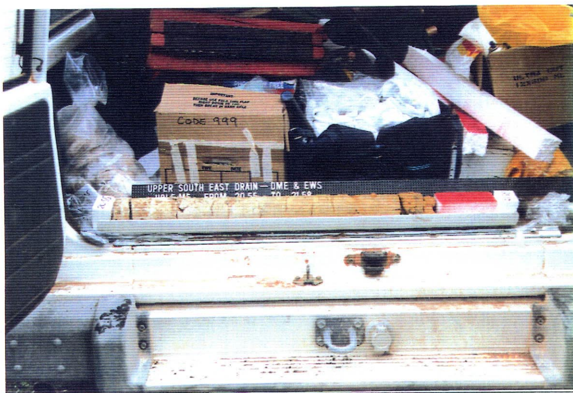
PLATE 23: SITE 2, Borehole M5. Core sample from 20.55 m to 21.58 m depth Photo No 40305
