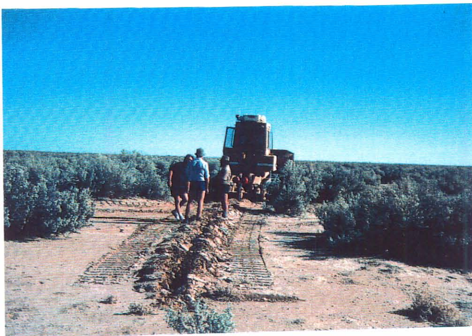
PLATE 3: Bulldozer ploughing in the geoflex detonating cord during the experimental work near Moppa Collina Channel. Note that the dozer blade is raised to avoid uprooting the salt bush vegetation.
