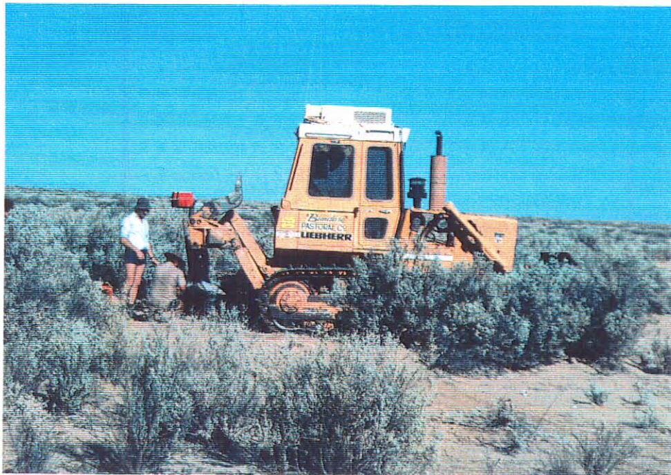
PLATE 2: Bulldozer with Geoflex cord spool/feeder assembly and hydraulic ripper tynes. The vegetation here is 'old man' salt bush.
