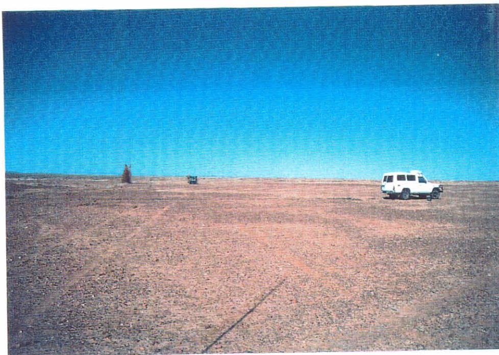
PLATE 4: Firing a shot, the shot man's vehicle (green) near the charge and the recording vehicle (white to the RHS).
