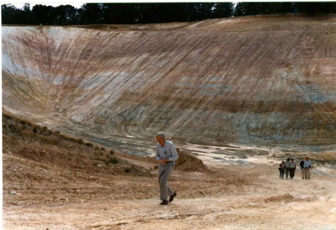
Plate C3. Selkirk Brick Pty Ltd, Ballarat North pit showing deeply weathered Ordovician shale used as a non-plastic component of brick clay blends. Neg. No. 39501
