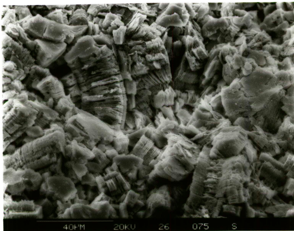
Plate 5. Scanning electron micrograph of coarse stacks of kaolinite crystals from the shaft sample. Photo No. 38898
