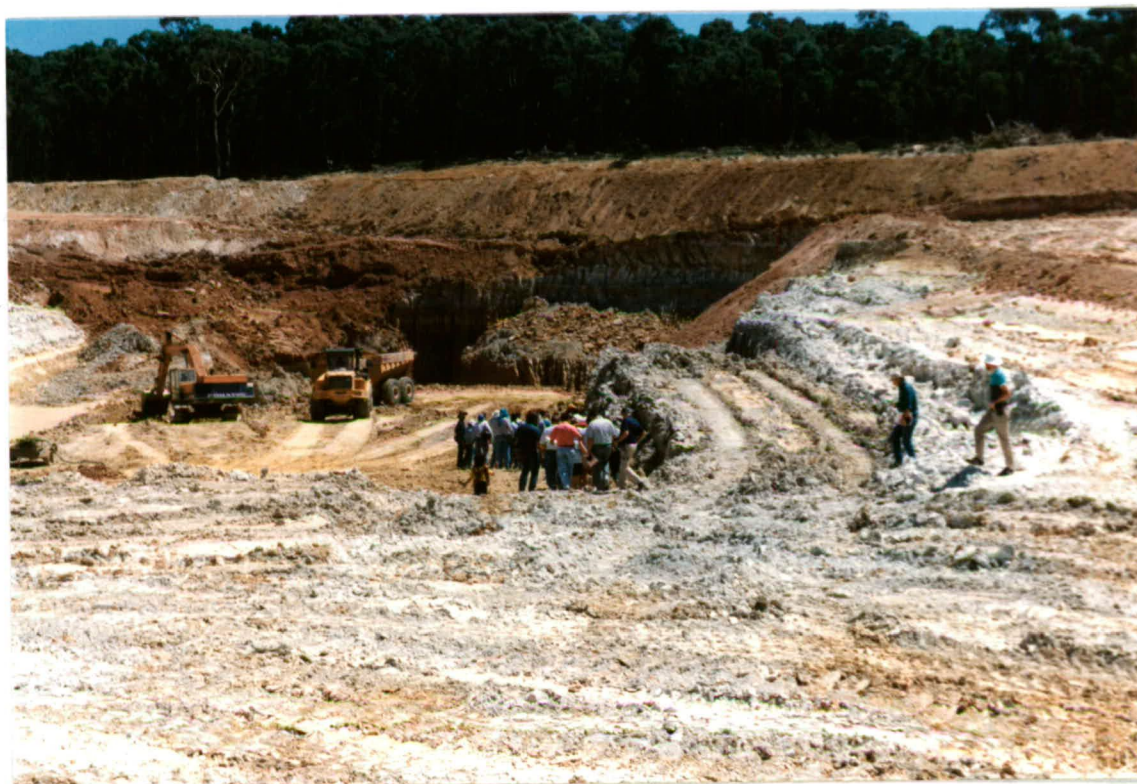
Plate C5. Enfield Clay Pit, 20 km south of Ballarat. Tertiary channel and swamp deposits are mined for pale and red burning semi-plastic clay for the brick and pipe industries.
