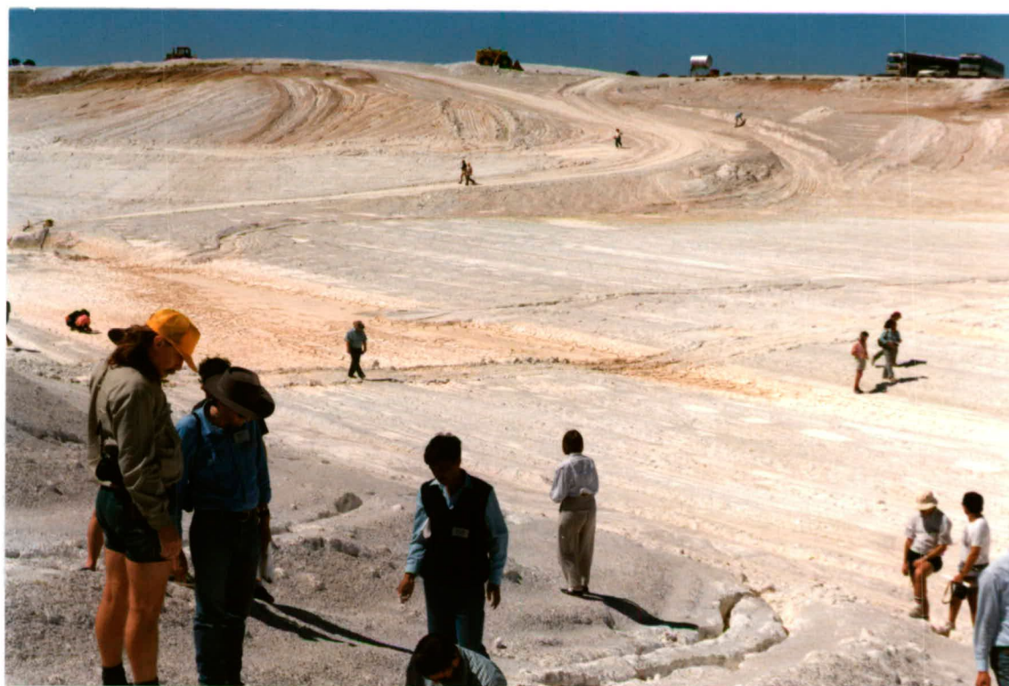
Plate D3. Pittong Kaolin Deposit (Kaolin Aust Pty Ltd). Kaolinized granodiorite which is mined by scraper and beneficiated on site to produce kaolin for the paper industry and for ceramics and general fillers. Feb. 1991.
