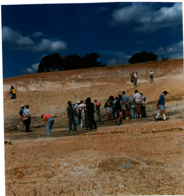
Plate C7. Buninyong Clay Pit, 3.5 km west of Buninyong. Tertiary montmorillonite/kaolin clay used as a 50% component in clay sewer pipe blends. Neg. No. 39505
