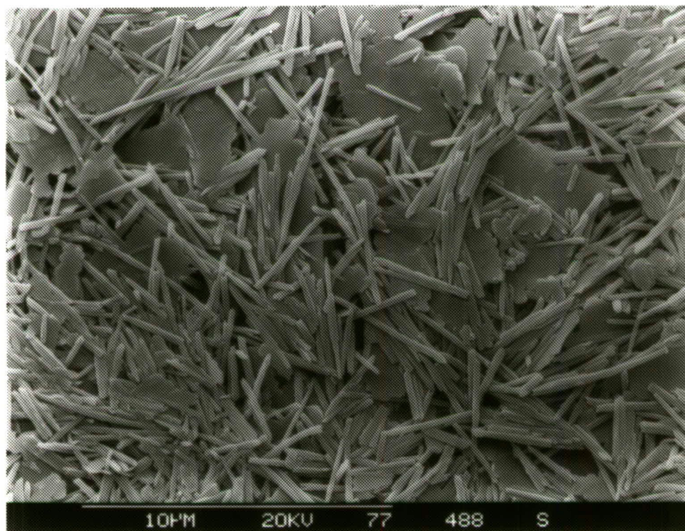
Plate 8. Dehydrated tubular halloysite in the <2\mu\text{m} fraction of a kaolin sample from hole MH 54.
