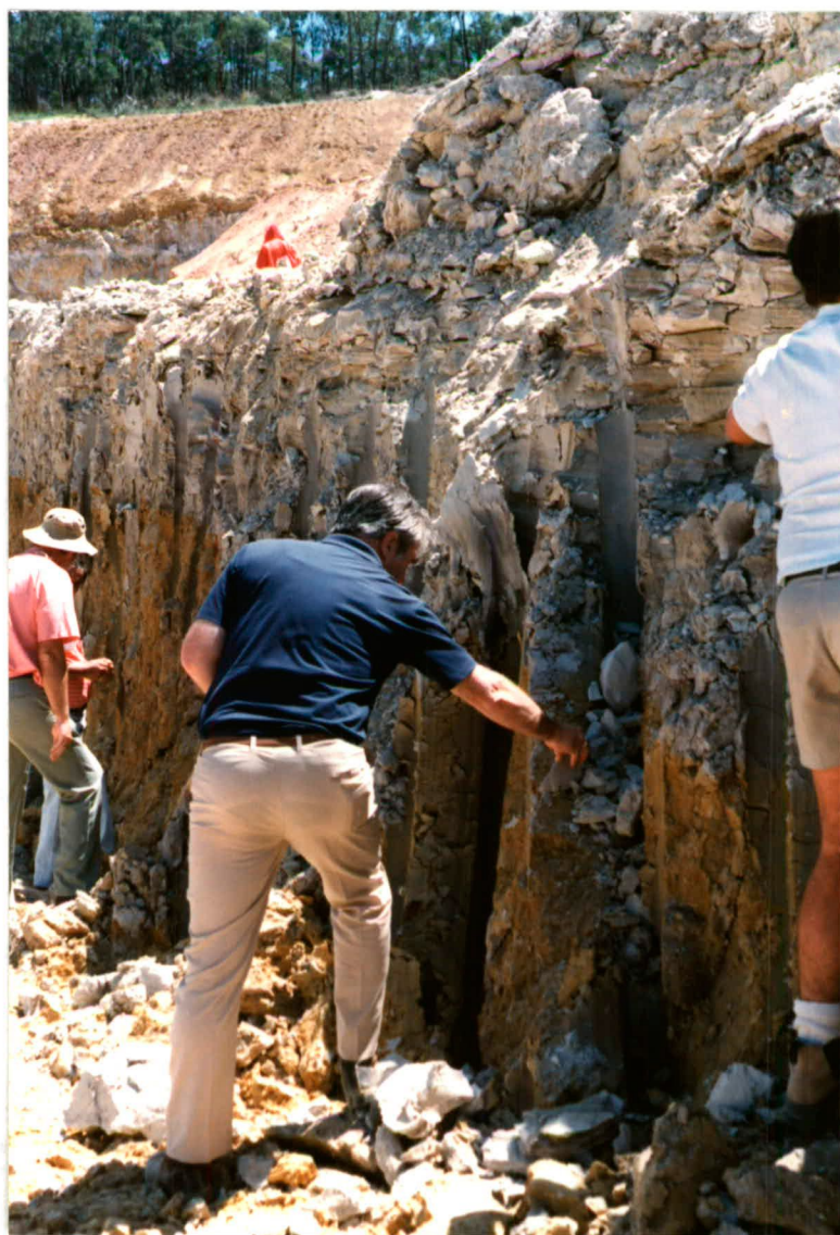
Plate C5. Enfield Clay Pit, 20 km south of Ballarat. Tertiary channel and swamp deposits are mined for pale and red burning semi-plastic clay for the brick and pipe industries.
