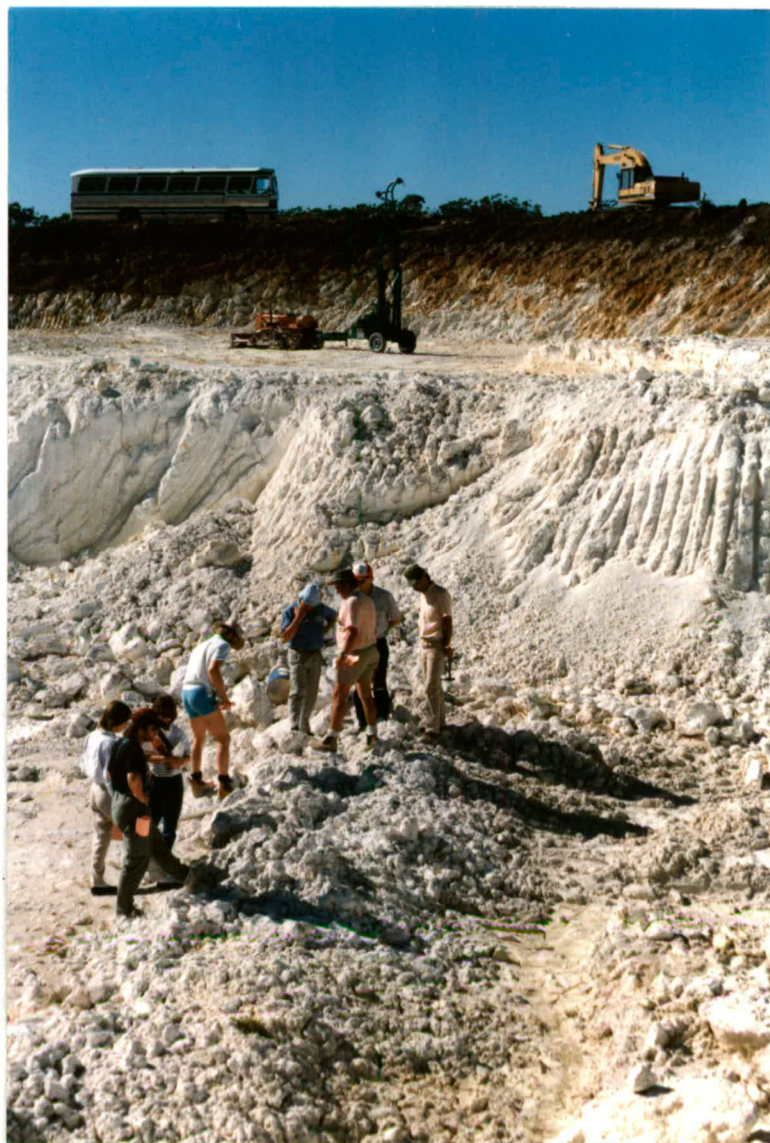
Plate D1. Lal Lal Kaolin Pit (Kaolin Aust. Pty Ltd) Peaty and clay soil overlying kaolinized granodiorite mined and processed for paper-coating and filler-grade kaolin. Feb. 1991.
