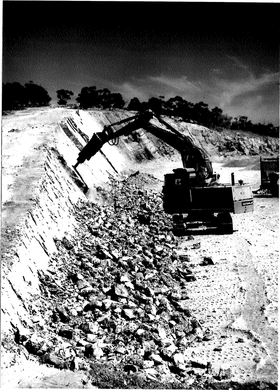
Plate 6. Mining of thin magnesite beds at Myrtle Springs. Neg. No. 38641
