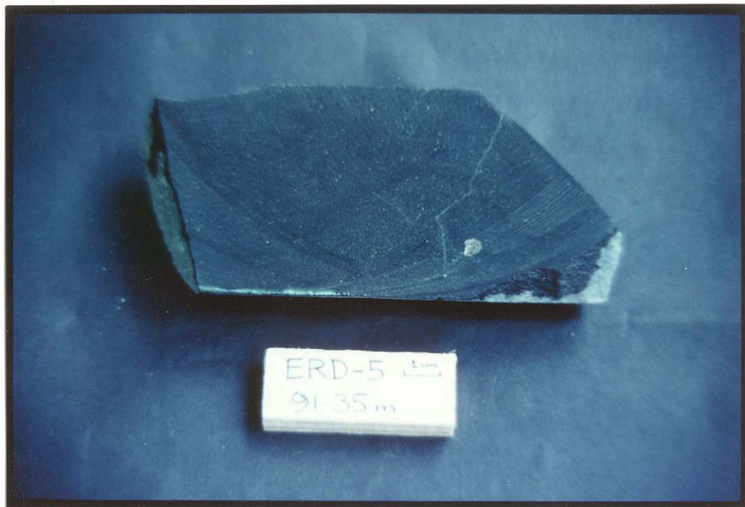
SLIDE 36458: ERD-5, 91.35 m. Blue-green, massive lithic sandstone of Labyrinth Formation. Pyrite aggregate lower right.
