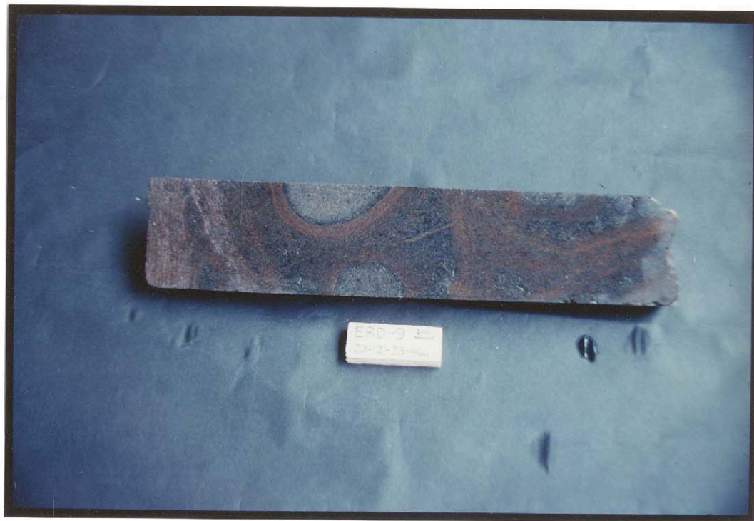
SLIDE 36461: ERD-9, 23.12-23.41 m. Dolerite of Gairdner Dyke Swarm. Note spheroidal weathering pattern.
