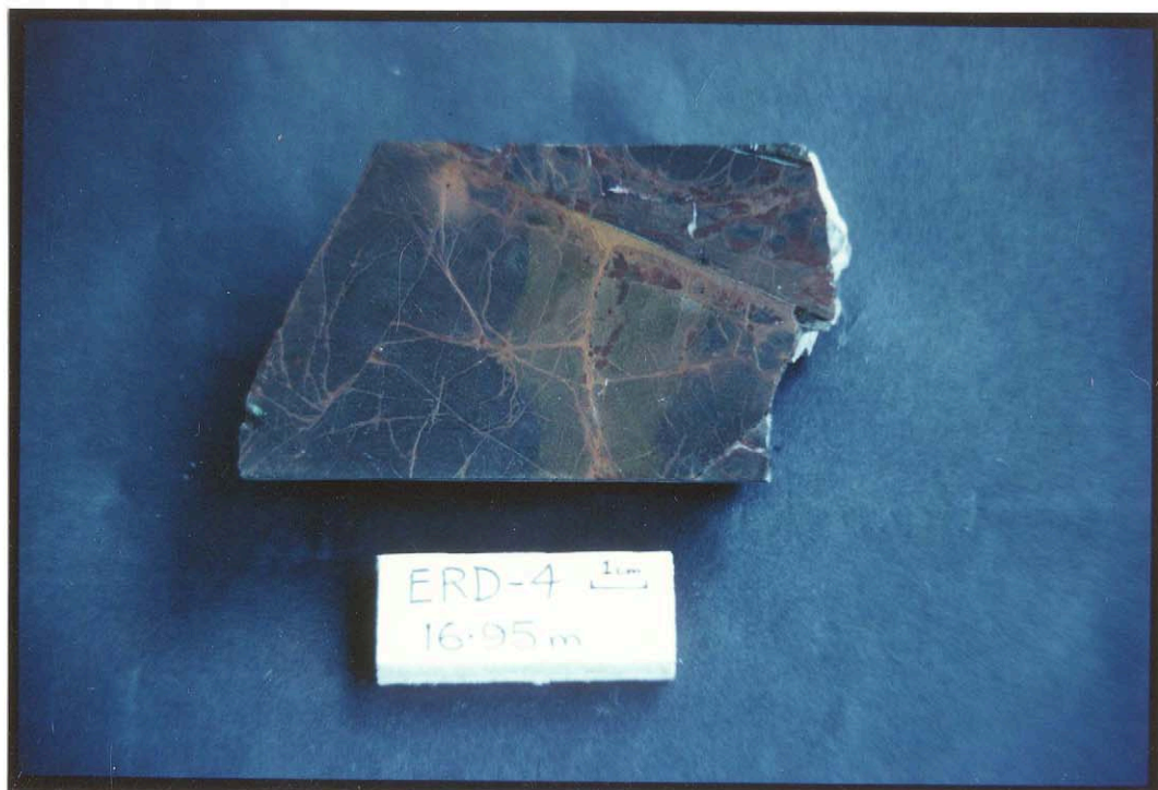
SLIDE 36457: ERD-4, 16.95 m. Massive dacite, Ealbara Rhyolite of Gawler Range Volcanics. Note orange and yellow alteration adjacent to fractures, and fine orange speckling.
