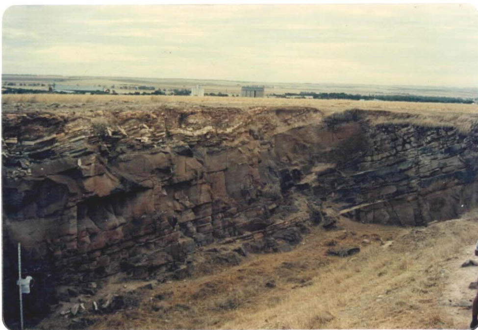
PLATE 4. NO. 3 QUARRY - VIEW NORTH WEST Basal sandstone Unit 1 at right overlain by flaggy sandstone Unit 2 about 1 m thick, thickly bedded building stone Unit 3, 1-2.5 m thick, and ochreous flaggy sandstone Unit 4, 0-1.5 m thick. Gladstone township in background. February 1984. Slide No. 36006
