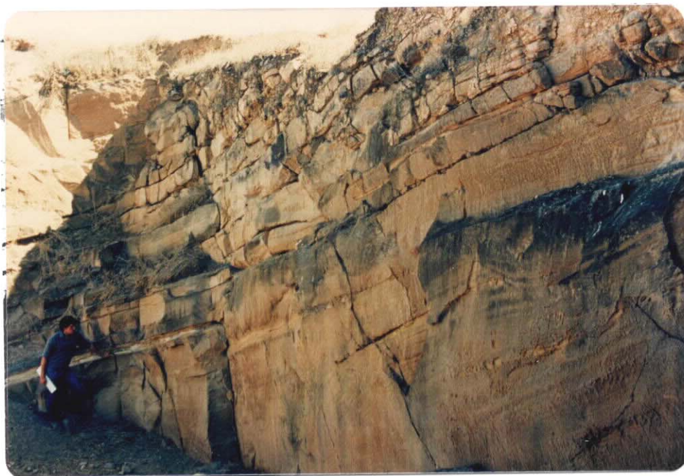
PLATE 5. NO. 3 QUARRY - TERMINAL FACE Thickly bedded basal sandstone Unit 1 to 2 m thick at right suitable for building stone. Top marked at left by yellow-white lens of fine-grained ochreous sandstone, 0.15 m thick. Some building stone is available from the overlying flaggy sandstone Unit 2. February 1984. Slide No. 36007
