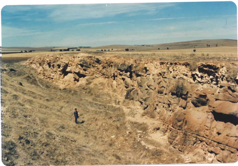
PLATE 3. NO. 3 QUARRY - VIEW SOUTH EAST Thickly bedded building stone Unit 3, 3 m thick in centre of face at right. Floor overgrown. Quarry 4 obscured in cropped paddock left rear in front of trees and farmhouse. February 1984 Slide No. 36005
