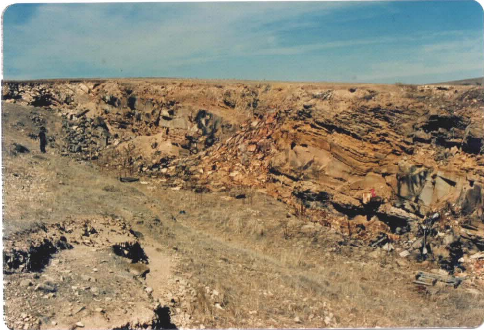
PLATE 2. NO. 2 QUARRY - VIEW SOUTH EAST Thickly bedded building stone Unit 3, 1-2 m thick in middle of face underlain by flaggy sandstone Unit 2 and overlain by ochreous sandstone Unit 4. Bedding is crenulated at top of Unit 3 at right centre. February 1984. Slide No. 36004
