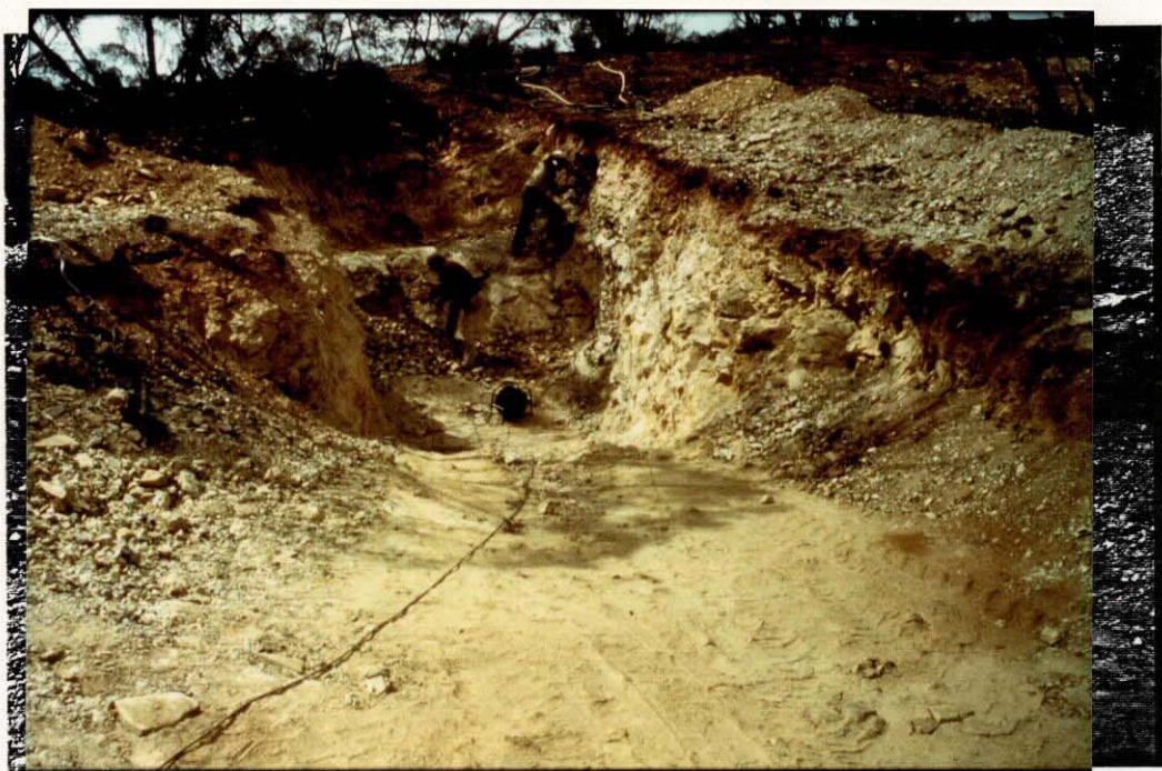
PLATE 8. No. 2 Open Cut. Channel sampling quartz veins using a Kango Hammer. Slide No. 36062
