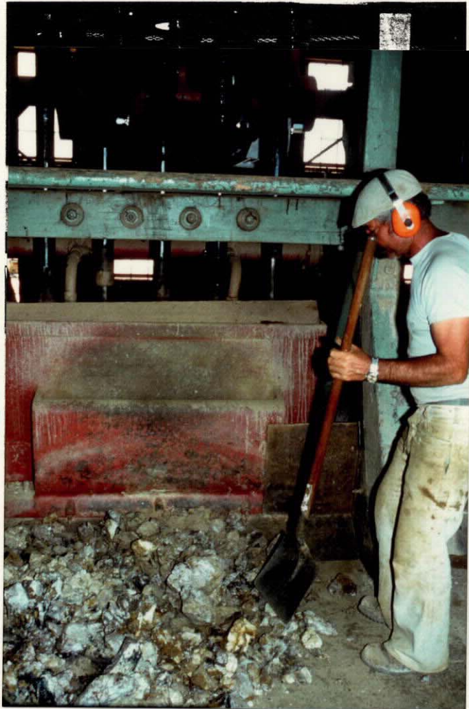
PLATE 12. Mount Grainger Ore from No. 2 Open Cut being fed to battery box at Peterborough State Battery. Slide No. 36066
