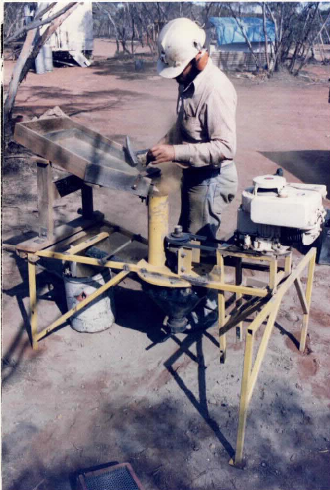
PLATE 10. Portable Crusher used to prepare samples prior to splitting for size analysis duplicate assaying.
