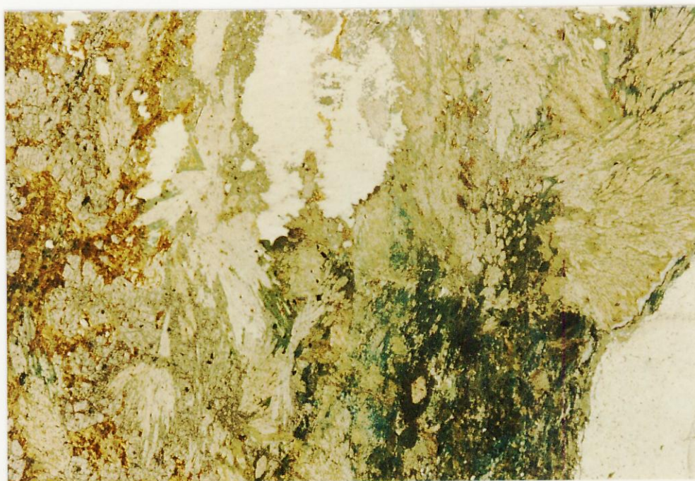
Plate 6. 6131 RS101, 427.6 m: Mount Shannan Iron Formation. Biotite + amphibole + garnet schist. Note intergrowth of actinolitic hornblende (green) and grunerite (pale fawn). Field of view 16 mm x 11 mm. (Plane polarised light)
