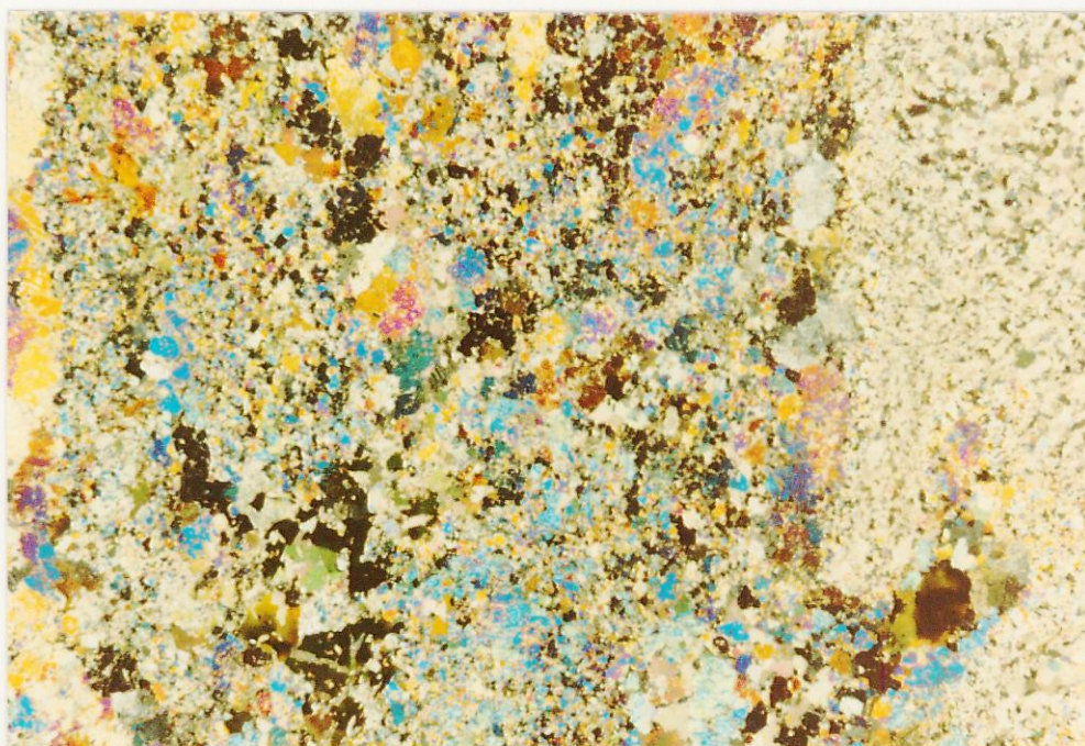
Plate 4. 6131 RS 122, 497.7 m: Mount Shannan Iron Formation. Medium-grained calcite + biotite + diopside gneiss. Note granoblastic texture. Field of view 16 mm x 11 mm. (Crossed nicols)
