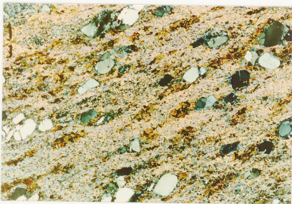
Plate 19. 6131 RS 76, 291.5 m: Bosanquet Formation. Fine- to medium-grained microcline + quartz + biotite + muscovite mylonitic rhyodacite. Note elongation lineation, defined by the preferred-dimensional orientation of relic quartz phenocrysts and biotite aggregate. Field of view 16 mm x 11 mm. (Crossed nicols)
