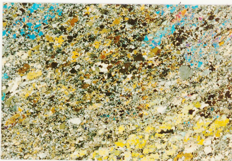
Plate 20. 6131 RS 74, 188.95: Bosanquet Formation. Quartz + microcline+diopside calcsilicate. Note granoblastic-elongate texture and optically - continuous relics of originally coarse-grained diopside. Compare with calcsilicates of the Mt Shannan Iron Formation (Plate 4). Field of view 16 mm x 11 mm. (Crossed nicols)
