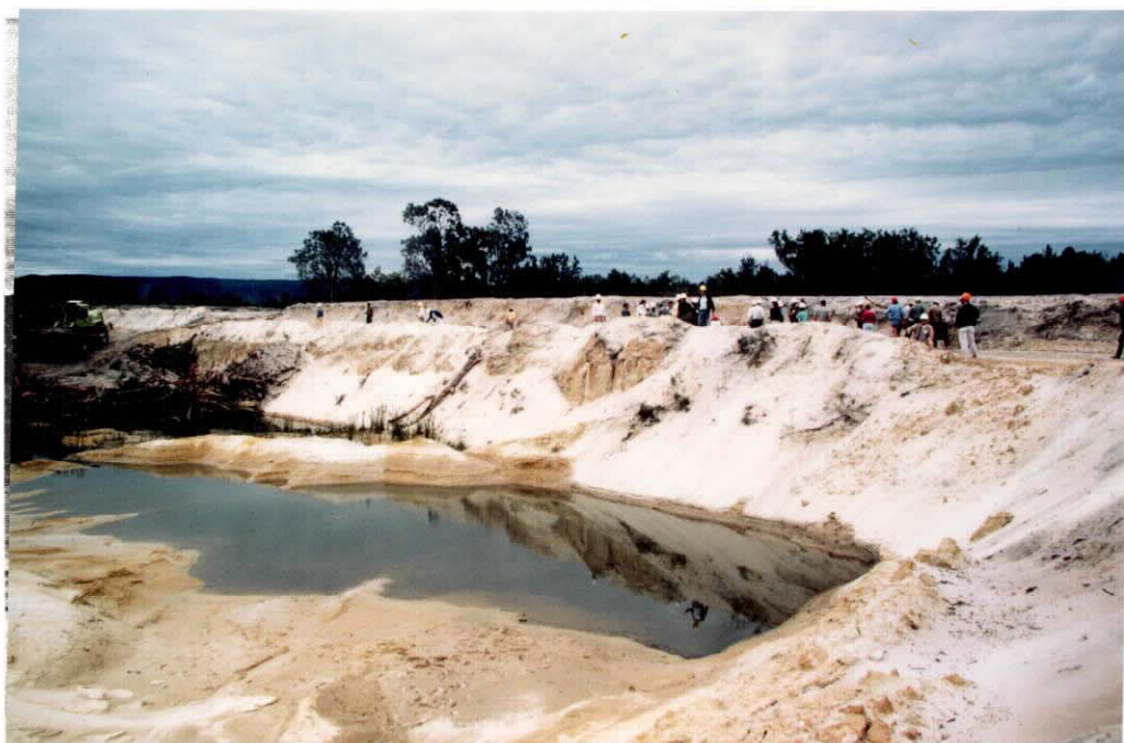
PLATE 14. LONDONDERRY SAND PIT, LONDONDERRY, N.S.W. Readymix-Farley sand pit showing area cleared of vegetation ready for mining. Agnes Bank Sand of (?)Tertiary age comprises clean, white, medium grained sand grading down into yellow, clayey sand. Sand is washed to produce construction sands. DECEMBER, 1986. SLIDE NO. 35806
