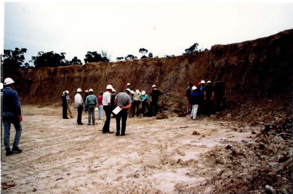
PLATE 13. LONDONDERRY CLAY PIT, LONDONDERRY, N.S.W. Sandy, silty, iron mottled, partly plastic Londonderry Clay of Tertiary age used in small quantities for brick and tile manufacture. DECEMBER, 1986. SLIDE NO. 35805
