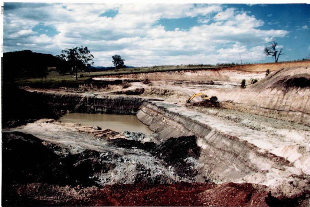
PLATE 17. CRESSFIELD BENTONITE DEPOSIT, northern Hunter Valley, N.S.W. General view north. Excavator is mining bentonite seam I (0.7 m thick). DECEMBER, 1986. SLIDE NO. 35809
