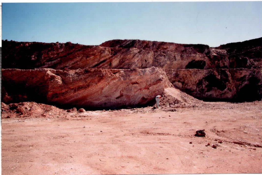
PLATE 19. WINGEN CHAMOTTE QUARRIES, Burning Mountain, northern Hunter Valley, N.S.W. Quarry No. 7 - halloysite quarry, view north. Burning of coal seam (right of photo) calcined kaolin flint clay to metakaolin, which has been rehydroxylated by ground water to halloysite. Used for low grade industrial absorbent. DECEMBER 1986. SLIDE NO. 35811
