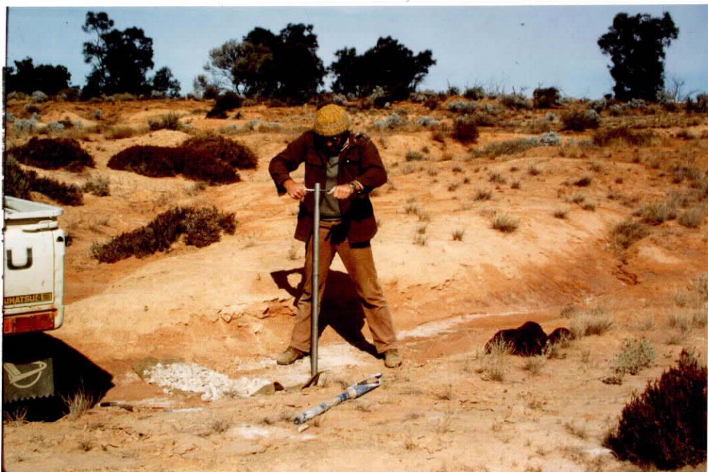
PLATE 8. HAND AUGERING - GARFORD FORMATION, COOBER PEDY. Obtaining samples for absorbancy testing. JUNE 1982. SLIDE NO. 24440.
