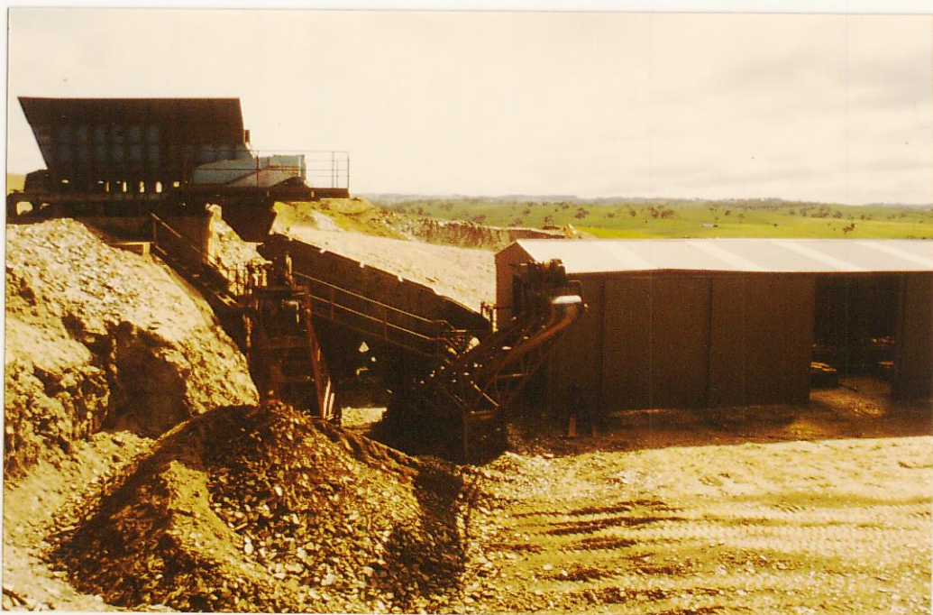
PLATE 9. Wistow No. 3 Quarry. View of apron feeder, vibrating screen and shed containing sorting belt. Quarry in background. Slide No. 35437.
