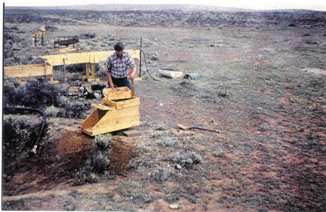
PLATE 45. SADME Alluvial Gold Treatment Equipment Display at Teetulpa Goldfield Centenary. Rocker in fore- ground, Long Tom, Dry Blower and Dry Shaker. October 1986. Slide No. 35570
