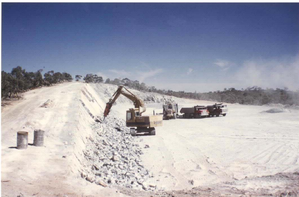
PLATE 4 Myrtle Springs magnesite open cut. Mechanised pneumatic rock breaker working one of a series of steep magnesite beds. December 1984. Slide No. 34407
